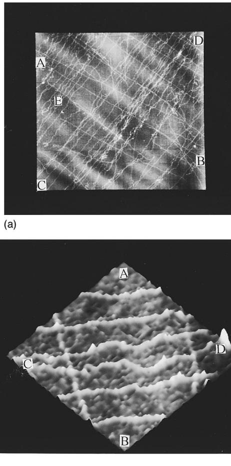
FIG. 1. AFM images of one-dimensional DNA strands aligned on the APS film surface by applying a molecular combing technique. (a) Scanning range:  $10\ \mu\text{m}\times 10\ \mu\text{m}$ ,  $z$  range: 0–2 nm (b) DNA strands on APS film with flaws. Scanning range:  $1.1\ \mu\text{m}\times 1.1\ \mu\text{m}$ , the  $z$  range: 0–6 nm.
