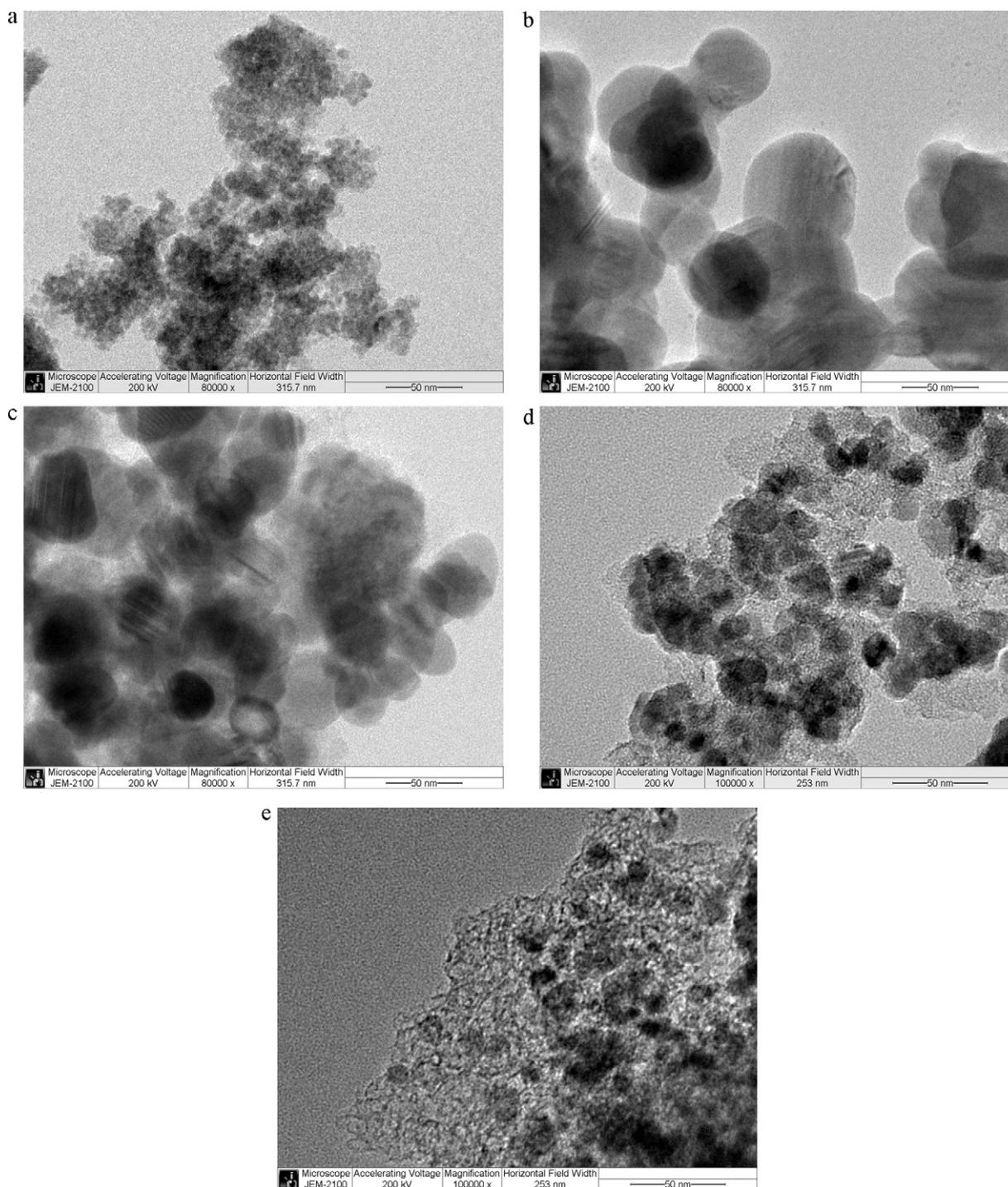
**Fig. 1.** TEM images of ZnS and ZnS/C composites: (a) dried ZnS precipitate, (b) bare ZnS, (c) ZnS/C (4.6 wt% C), (d) ZnS/C (9.3 wt% C) and (e) ZnS/C (11.4 wt% C).
