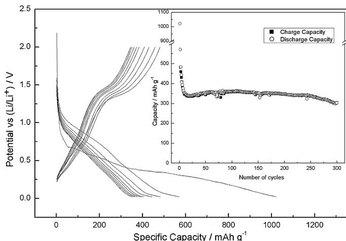
**Fig. 4.** Charge and discharge profiles and the cycling performance of ZnS/C (9.3 wt% C) electrode at the specific current of 400 mA/g.
