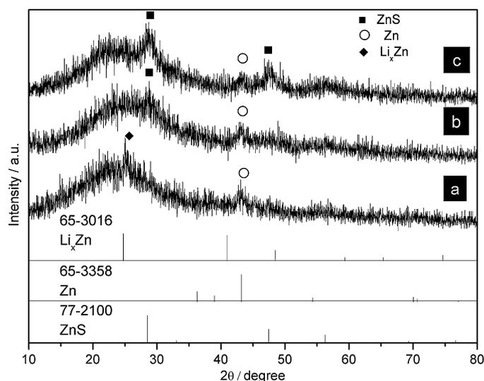
**Fig. 10.** Ex situ XRD patterns of ZnS/C electrode during the first cycle at different charge potentials (a: 0.05 V, b: 1.4 V, c: 2.0 V).
