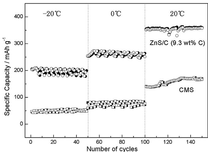
**Fig. 7.** Cycling performance of ZnS/C (9.3 wt% C) anode and commercial MCMB anode at wide-ranging temperature with a charge–discharge specific current of 400 mA/g.
