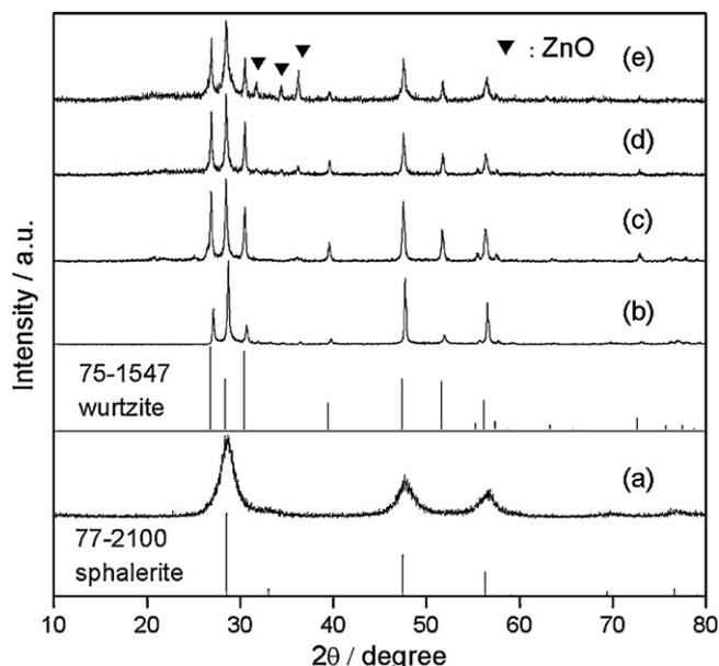
Fig. 2. XRD patterns of ZnS and ZnS/C composites: (a) dried ZnS precipitate, (b) bare ZnS, (c) ZnS/C (4.6 wt% C), (d) ZnS/C (9.3 wt% C) and (e) ZnS/C (11.4 wt% C).
