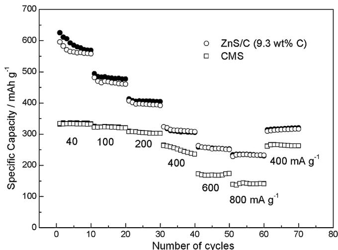
**Fig. 6.** Comparison of rate capability of the ZnS/C (9.3 wt% C) anode and commercial MCMB anode with a charge–discharge specific current range from 40, 100, 200, 400, 600 to 800 mA/g.
