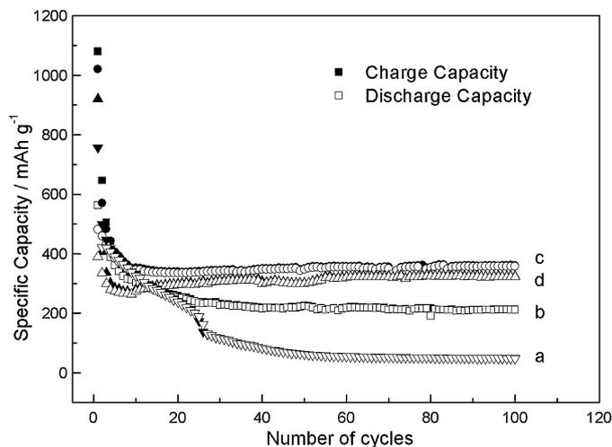
Fig. 3. Cycling performance of the various ZnS/C composites with different carbon contents at the specific current of 400 mA/g. (a) bare ZnS, (b) ZnS/C (4.6 wt% C), (c) ZnS/C (9.3 wt% C) and (d) ZnS/C (11.4 wt% C).
