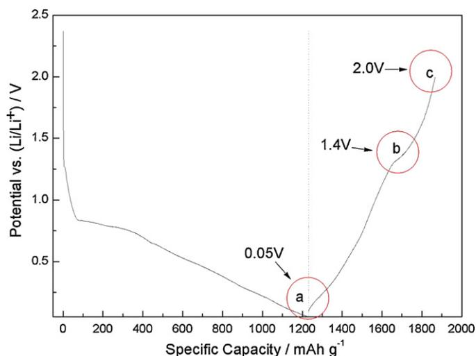
**Fig. 9.** First discharge and charge profile of ZnS/C electrode at the specific current of 40 mA/g.
