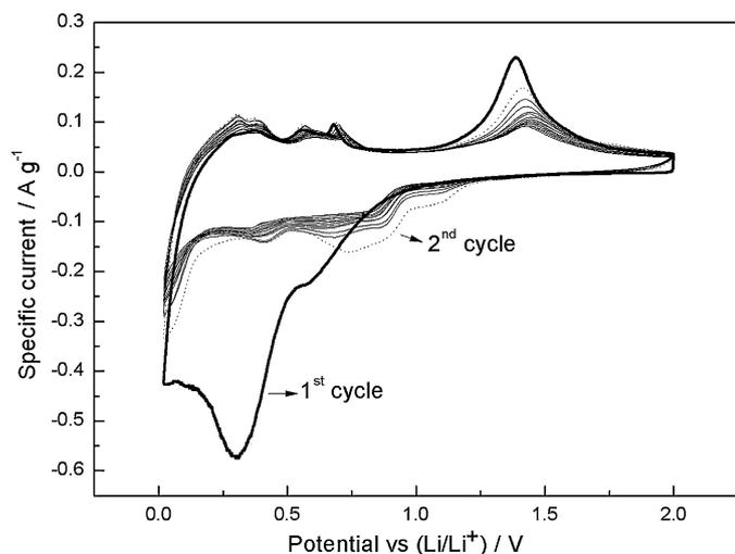
**Fig. 5.** Cyclic voltammograms of the ZnS/C (9.3 wt% C) electrode at a scan rate of 0.1 mV/s.
