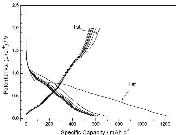
**Fig. 8.** Discharge and charge profiles and the cycling performance of ZnS/C at the specific current of 40 mA/g.
