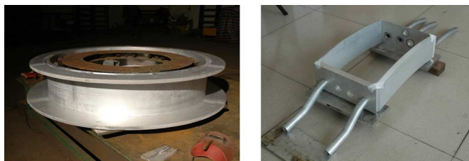
Fig. 5. Mandrel after welding, pre-assembly of cooling tubing and He vessel.
