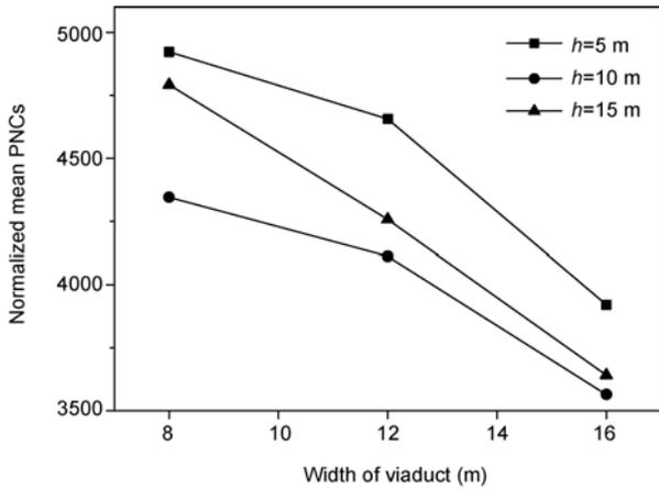
**Figure 5** The mean particles number concentrations in street canyons with a viaduct (dash line: the mean PNCs in case 1).
