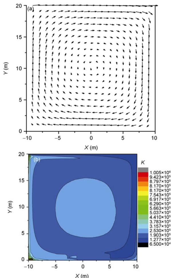
**Figure 2** (a) Mean velocity vectors; (b) distribution of normalized concentrations.
