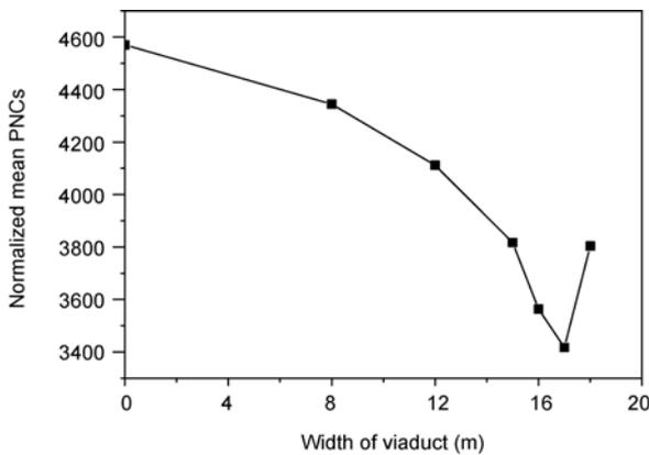
**Figure 6** The mean PNCs in street canyons with different width viaducts when *h* is 10 m.
