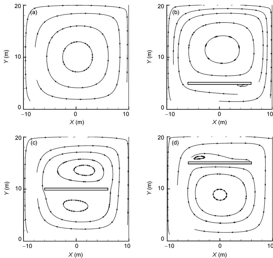
**Figure 4** The stream lines in street canyons with viaduct at different heights above ground. (a) Case 1; (b) case 3; (c) case 6; (d) case 9.
