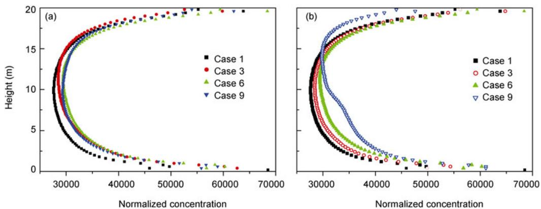
**Figure 7** Vertical profiles of the normalized PNCs at wall A. (a) Street canyons with a 12 m-width viaduct; (b) street canyons with a 10 m-height viaduct.
