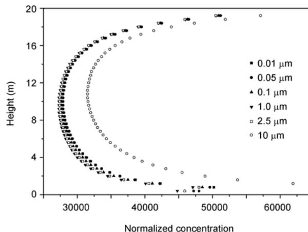
**Figure 3** Particles number distributions at wall A in case 1 with different aerodynamic diameters.
