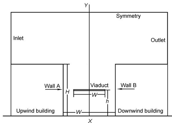
Figure 1 Schematic diagram of street canyon with a viaduct.
