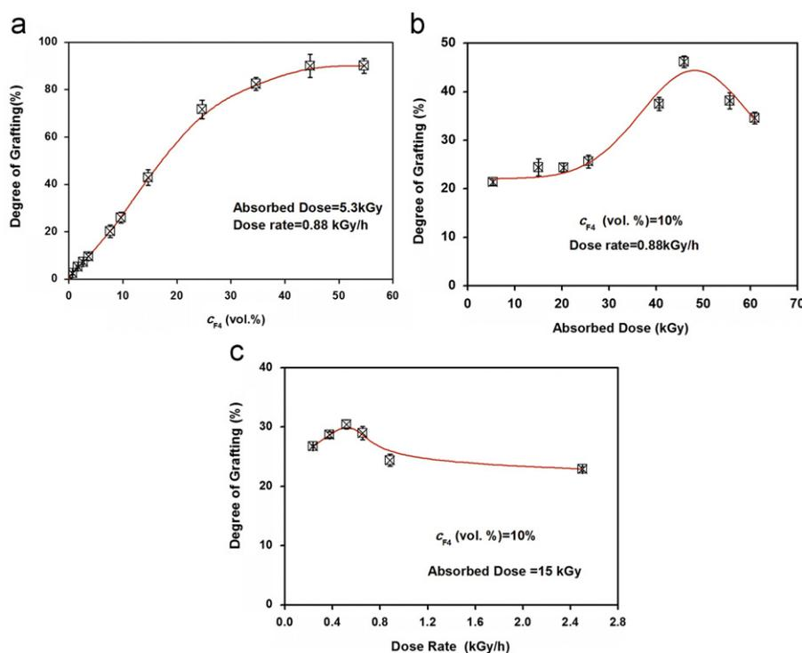
**Fig. 1.** Kinetic study result of the relationship between the DG and the experimental parameters of (a) concentration of F4 at dose rate of 0.88 kGy/h and total absorbed dose of 5.3 kGy, (b) absorbed dose at  $c_{F4}$  of 10% and dose rate of 0.88 kGy/h and (c) dose rate at  $c_{F4}$  of 10% and total absorbed dose of 15 kGy.
