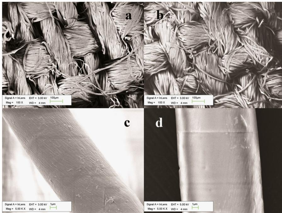
Fig. 2. Low range SEM image (magnified to  $100\times$ ) of (a) the pristine cotton fabric and (b) the cotton-F4 with a DG of 28%. The SEM image of (c) a single fabric of the pristine cotton fabric and (d) a single fabric of the cotton-F4 with a DG of 28%.
