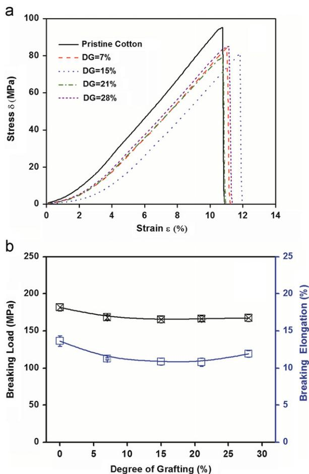
Fig. 3. Mechanical properties of the fabrics: (a) the relationship between stress and strain of the pristine cotton fabric and cotton-F4 with different DG ( $\delta \sim \epsilon$ ), and (b) the breaking load and breaking elongation of the pristine cotton fabric and cotton-F4 with different DG.
