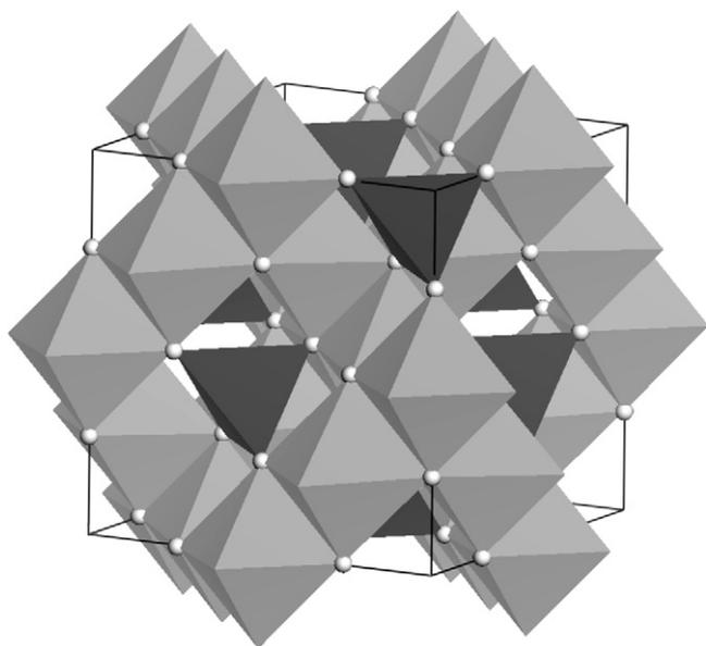
Fig. 1. The unit cell of magnetite.
