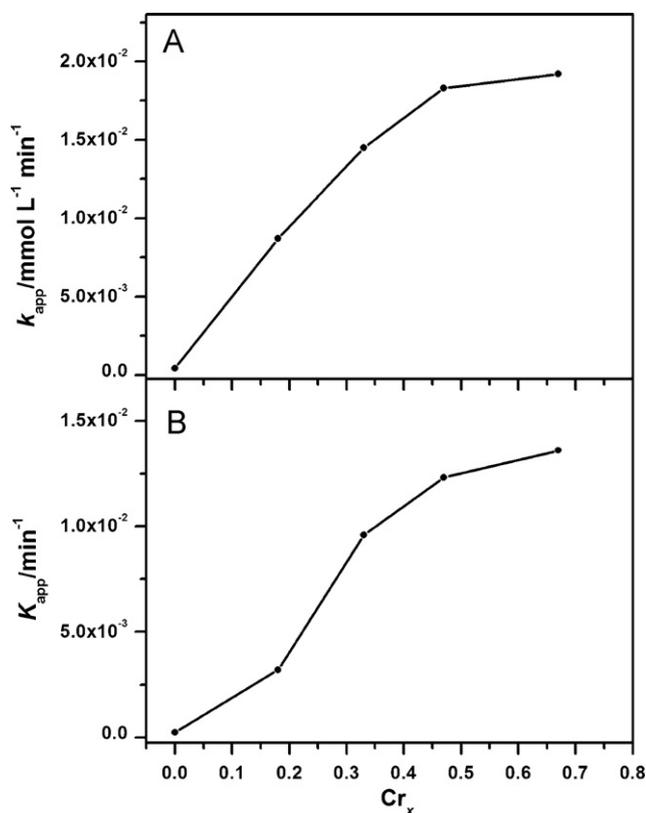
Fig. 10. Degradation rate constants for the degradation of (A) methylene blue and (B) acid orange II (second stage) with  $H_2O_2$  in the presence of  $Fe_{3-x}Cr_xO_4$ .
