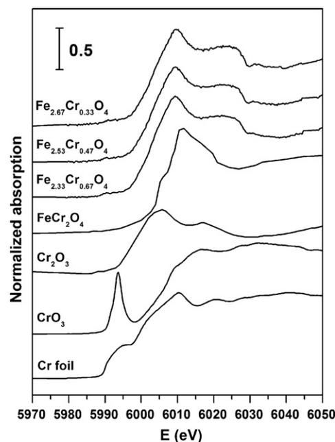
Fig. 4. Cr K-edge XANES spectra of Cr foil,  $Cr_2O_3$ ,  $CrO_3$ ,  $FeCr_2O_4$  and series  $Fe_{3-x}Cr_xO_4$ .
