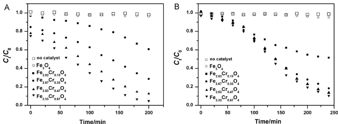
Fig. 6. Decolorization of (A) methylene blue and (B) acid orange II through heterogeneous Fenton reaction catalyzed by  $\text{Fe}_{3-x}\text{Cr}_x\text{O}_4$  ( $C_0 = 0.2 \text{ mmol L}^{-1}$ ,  $80 \text{ mmol L}^{-1}$  of  $\text{H}_2\text{O}_2$ ,  $1.0 \text{ g L}^{-1}$  of catalyst,  $250 \text{ mL}$ ,  $\text{pH } 7.0$ ,  $25^\circ \text{C}$ ).
