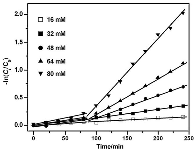
**Fig. 8.** Degradation of acid orange II through heterogeneous Fenton reaction by  $\text{Fe}_{2.33}\text{Cr}_{0.67}\text{O}_4$  with different  $\text{H}_2\text{O}_2$  concentrations ( $C_0 = 0.2 \text{ mmol L}^{-1}$ ,  $1.0 \text{ g L}^{-1}$  of  $\text{Fe}_{2.33}\text{Cr}_{0.67}\text{O}_4$ , 250 mL, pH 7.0,  $25^\circ\text{C}$ ).
