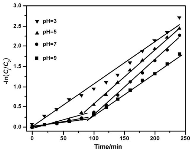
**Fig. 9.** Degradation of acid orange II through heterogeneous Fenton reaction by  $\text{Fe}_{2.33}\text{Cr}_{0.67}\text{O}_4$  at different initial pH ( $C_0 = 0.2 \text{ mmol L}^{-1}$ ,  $80 \text{ mmol L}^{-1}$  of  $\text{H}_2\text{O}_2$ ,  $1.0 \text{ g L}^{-1}$  of  $\text{Fe}_{2.33}\text{Cr}_{0.67}\text{O}_4$ , 250 mL,  $25^\circ\text{C}$ ).
