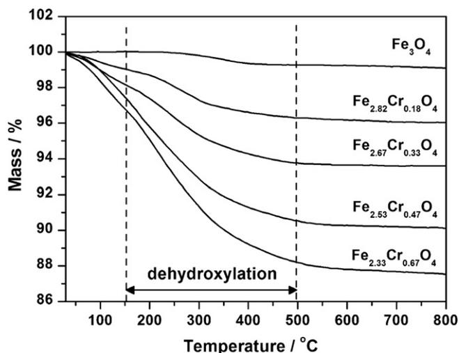
Fig. 5. Thermogravimetric profiles of  $\text{Fe}_{3-x}\text{Cr}_x\text{O}_4$  samples under  $\text{N}_2$ .
