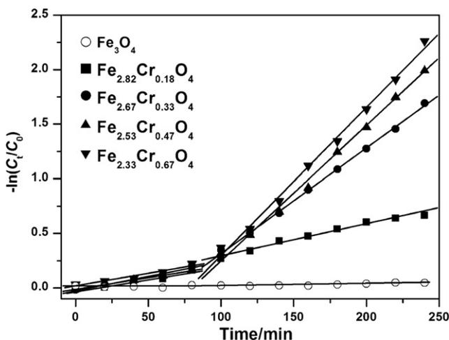
**Fig. 7.** Kinetics fitting of the acid orange II decolorization through heterogeneous Fenton reaction catalyzed by  $\text{Fe}_{3-x}\text{Cr}_x\text{O}_4$  ( $C_0 = 0.2 \text{ mmol L}^{-1}$ ,  $80 \text{ mmol L}^{-1}$  of  $\text{H}_2\text{O}_2$ ,  $1.0 \text{ g L}^{-1}$  of catalyst, 250 mL, pH 7.0,  $25^\circ\text{C}$ ).
