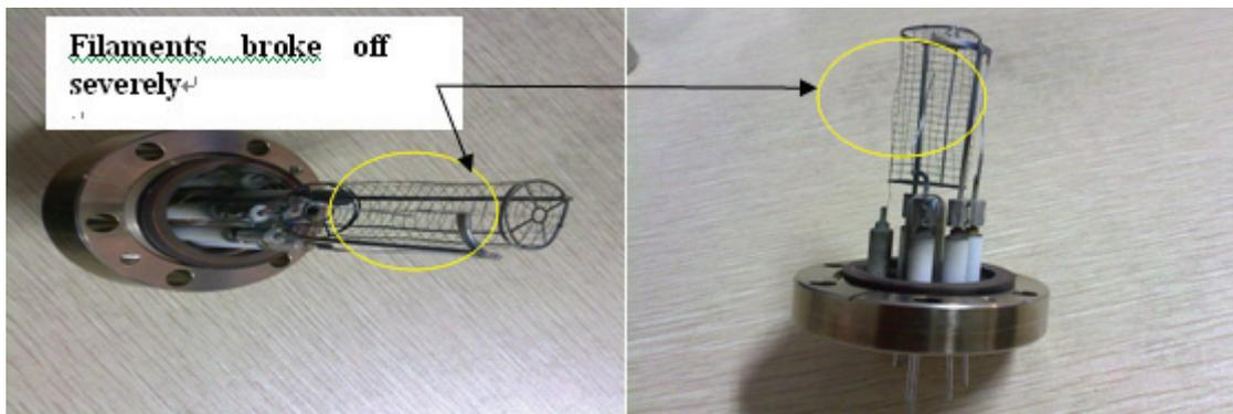
**Fig 10 : Ionization vacuum gauge filaments break off**
