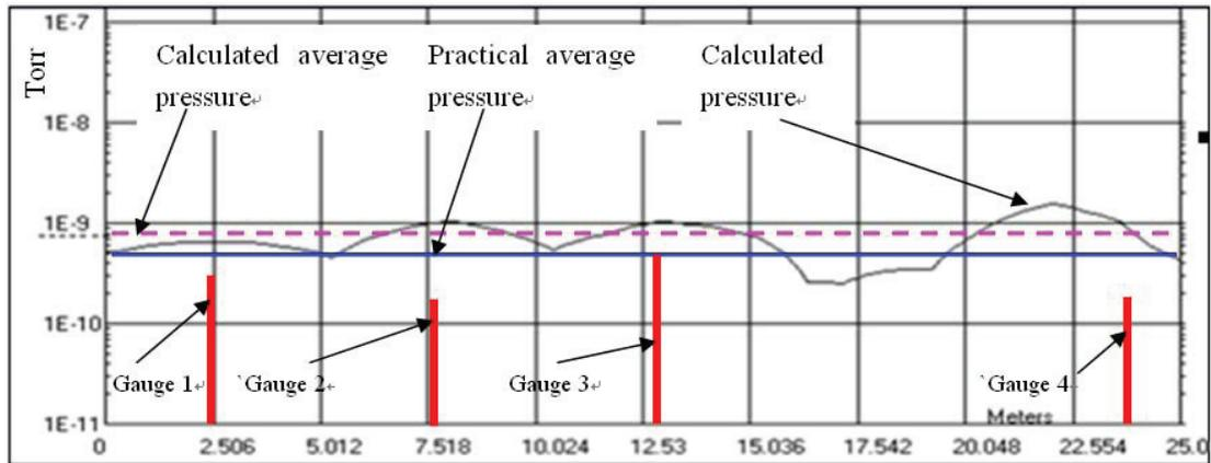
Fig 4 :Pressure Distribution in a Cell B
