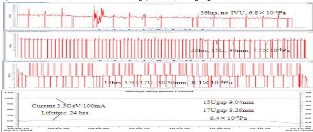
**Fig 6 : Relationship between Lifetime and Pressure and IVU Gap**
