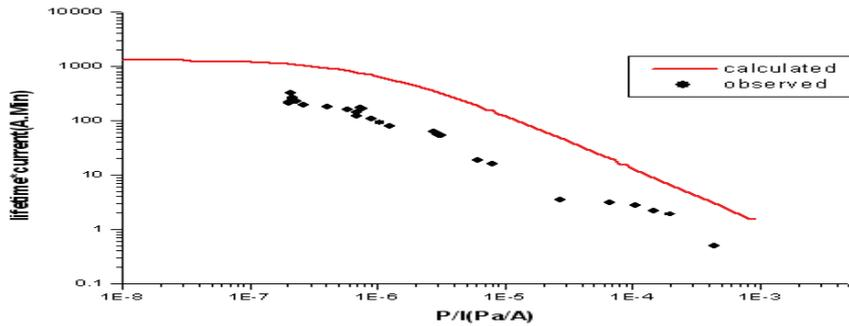
**Fig 7 : The influence of residual gases to beam lifetime**
