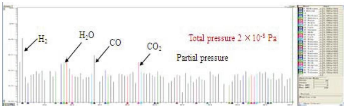
**Fig 2 :Total and Partial Pressure in the Ring without**
