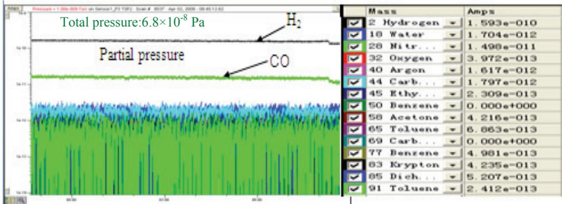
Fig 3 :Total and Partial Pressure in the Ring with Beam (3.5GeV/200mA)
