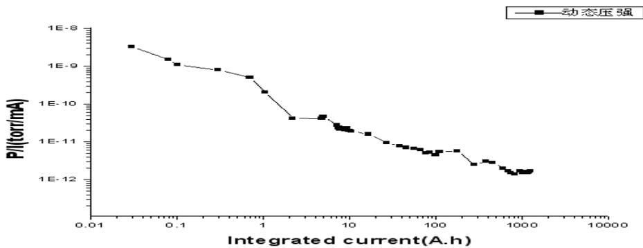
**Fig 8 :Relationship between Pressure  $P_{av}/I$  and Dose (0~1200Ah)**
