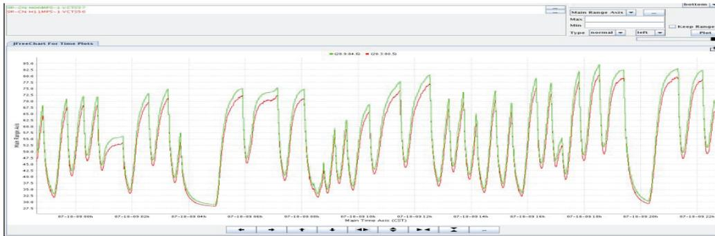
**Fig 9 :Temperature of vacuum chamber rise greatly somewhere**
