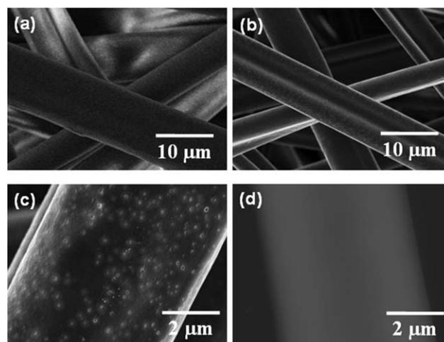
**Fig. 2** (a) FE-SEM images of the composite PS-PU fibers formed at (a) 20 and (b) 25 kV. (c) High magnification SEM image and (d) TEM image of the fiber formed at 25 kV. (A 20 wt% PS dissolved in 1 : 4 THF/DMF was used as the shell solution and the initial PU resin was used as the core solution.)
