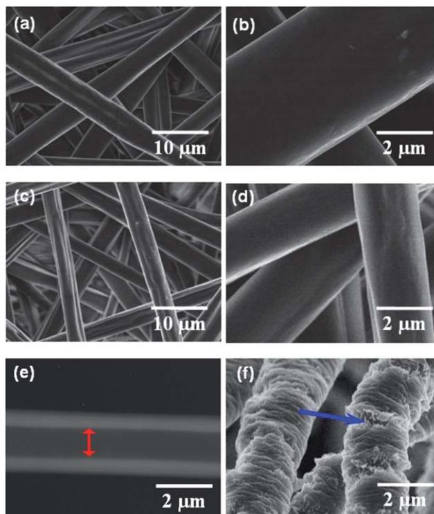
**Fig. 3** FE-SEM images of the composite PS–PU fibers formed with (a) 75 and (c) 50 wt% PU solutions as the core solutions. (b) and (d) show the high magnification images of the samples shown in (a) and (c), respectively. (e) TEM image of as-spun fiber shown in (c). (f) FE-SEM image of fibers shown in (c) after stretching. (A 20 wt% PS dissolved in 1 : 4 THF/DMF was used as the shell solution; the applied voltage was kept at 25 kV.)
