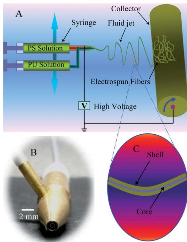
**Fig. 1** (A) Schematic representation showing the core–shell electrospinning setup used in this study. (B) Photograph of the co-axial spinneret. (C) An illustration of the electrospun core–shell fiber.
