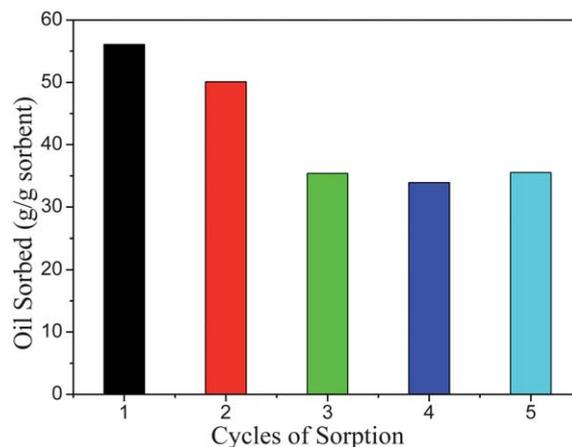
Fig. 11 Reusability of the composite PS-PU fibrous mat for motor oil.
