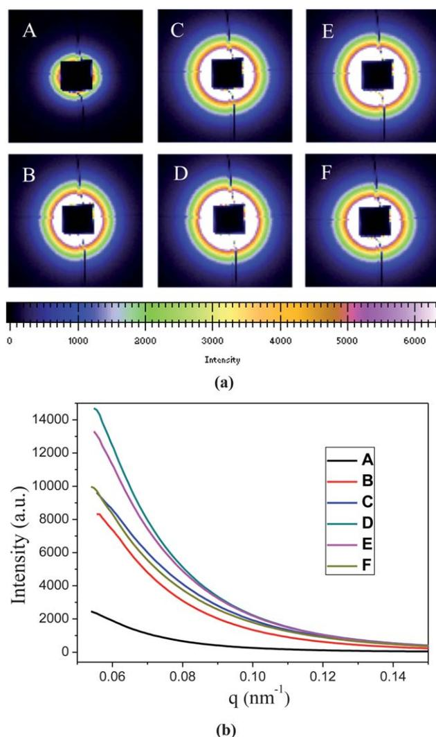
**Fig. 6** (a) SAXS 2D scattering patterns and (b) SAXS curves of the composite PS-PU fibrous mats. (The samples A to F are the corresponding fibers shown in Table 2. Fit2D software was used to analyze the 2D SAXS data.)
