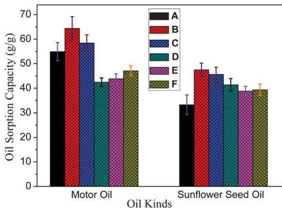
**Fig. 8** Sorption capacities of the composite PS-PU fibrous mats for motor oil and sunflower seed oil. (The samples A to F are the corresponding fibers shown in Table 2.)
