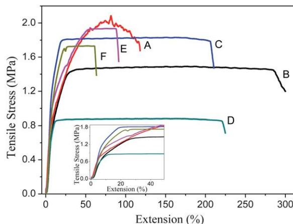
Fig. 12 Typical stress-strain curves for the composite PS-PU fibrous mats. (The samples A to F are the corresponding fibers shown in Table 2.)
