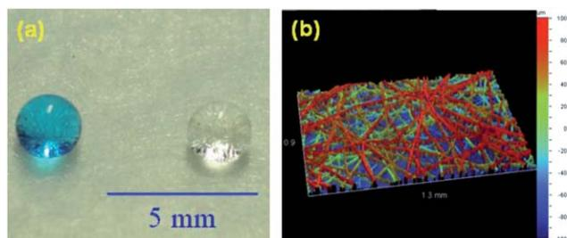
**Fig. 7** (a) Optical image of water droplets on the as-prepared fibrous mat. (b) Optical profilometry image of the as-prepared fibrous mat. The water was labeled with blue color.
