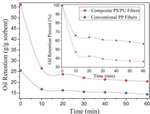
Fig. 10 Plot of oil retention on the composite PS-PU fibrous mats during free draining.
