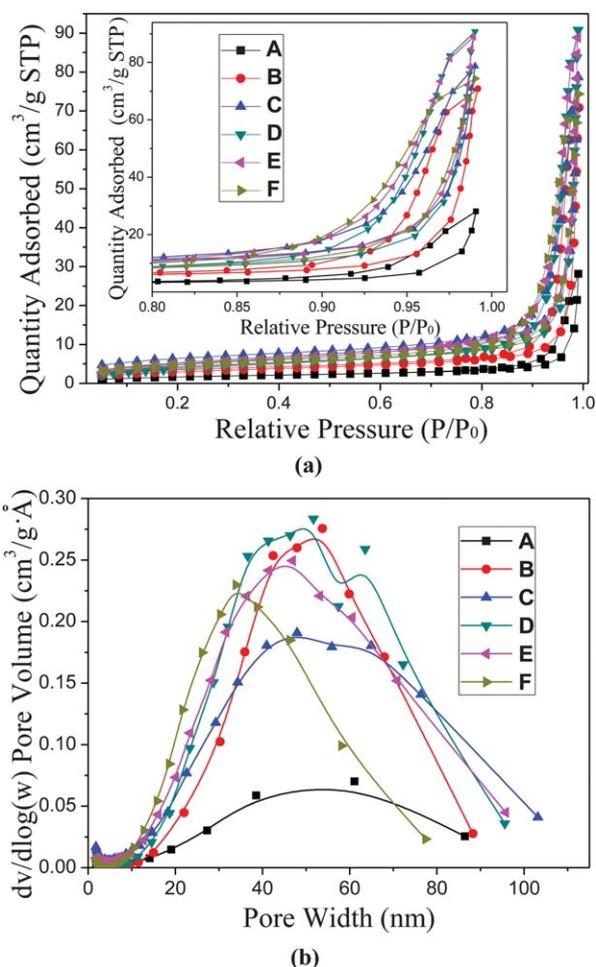
**Fig. 5** (a) Nitrogen adsorption-desorption isotherms of the composite PS-PU fibrous mats. (b) Pore size distribution curves of the composite PS-PU fibrous mats calculated from the desorption branch by using BJH method. (The samples A to F are the corresponding fibers shown in Table 2.)
