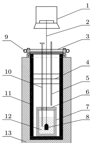
**Fig. 1.** Schematic diagram of the density measuring device: (1) electronic balance, (2) platinum wire, (3) brass lid, (4) heat insulation plate, (5) corundum inlet pipe for Ar gas, (6) crucible lid, (7) BN or graphite crucible, (8) platinum cylinder, (9) copper cooling pipe, (10) thermocouple, (11) corundum furnace tube, (12) molten salts, (13) thermal insulator.
