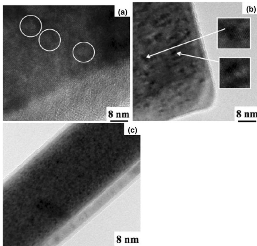
**Fig. 4** HRTEM images of the ZnO NWs irradiated by 70 keV  $Ar$  ions at room temperature at the doses of **a**  $1 \times 10^{15}$  ion/cm<sup>2</sup>, **b**  $5 \times 10^{15}$  ion/cm<sup>2</sup>, and **c**  $1 \times 10^{16}$  ion/cm<sup>2</sup>
