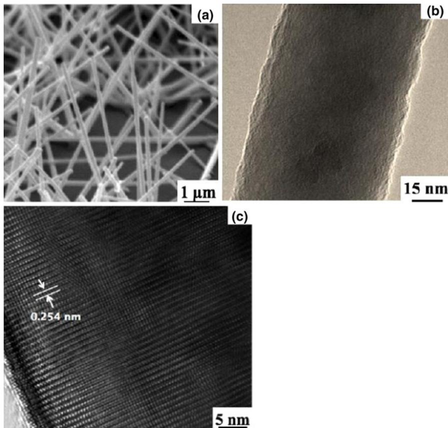
**Fig. 1** a SEM images of ZnO NWs arrays prepared by VTD method. b TEM image of ZnO nanowires. c HRTEM image of the nanowire
