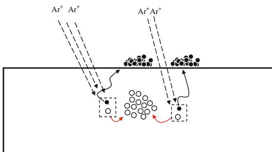
**Fig. 5** A schematic diagram showing the generation, migration, and accumulation of interstitials and vacancies in ZnO NW under irradiation of 70 keV  $\text{Ar}^+$  ion beam at room temperature
