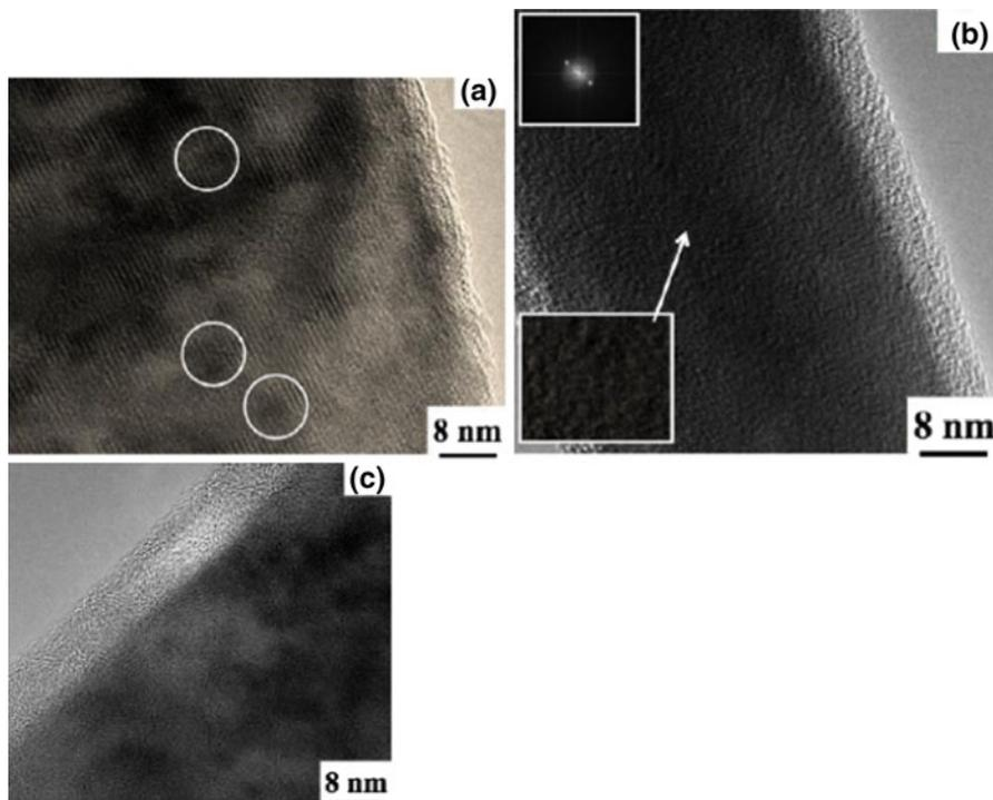
**Fig. 3** HRTEM images of the ZnO NWs irradiated by 70 keV  $N^+$  ion beam at room temperature at the doses of **a**  $1 \times 10^{15}$  ion/cm<sup>2</sup>, **b**  $1 \times 10^{16}$  ion/cm<sup>2</sup>, the *inset* is the corresponding SAED image. **c**  $5 \times 10^{16}$  ion/cm<sup>2</sup>
