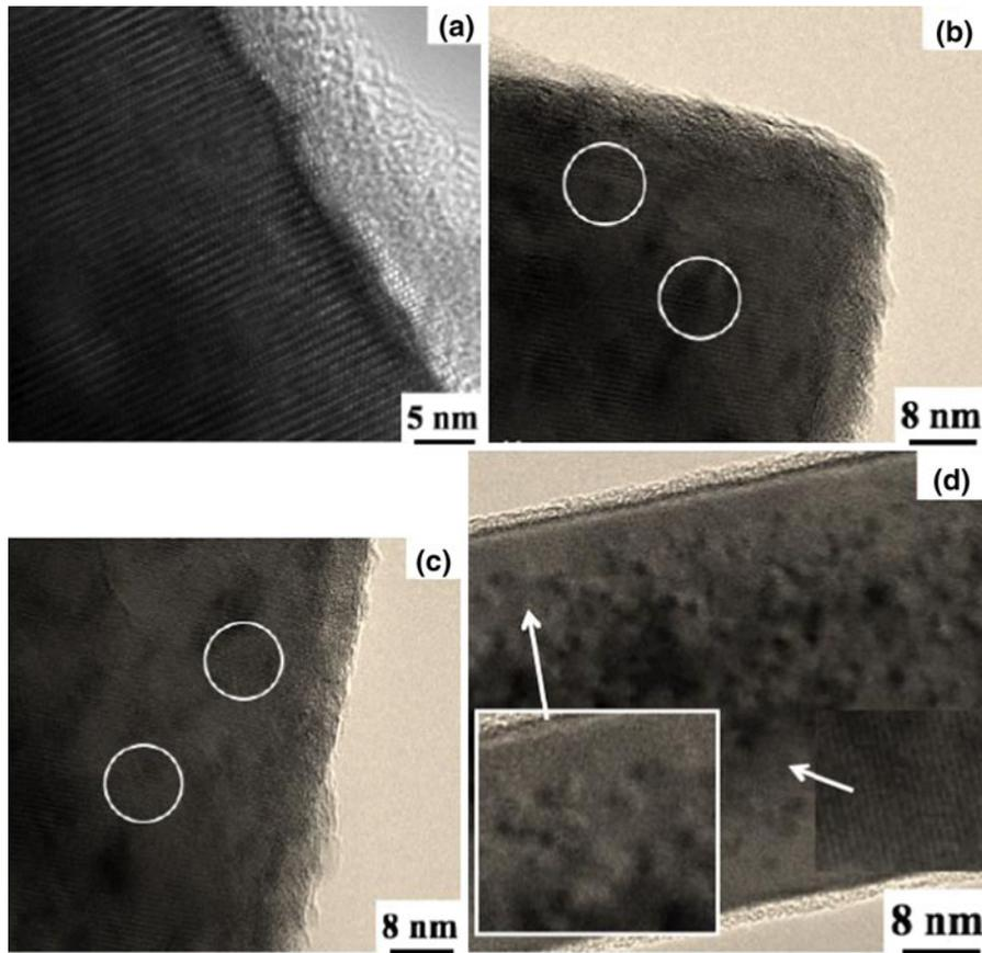
**Fig. 7** HRTEM images of the ZnO NWs irradiated by 70 keV at 400 °C at the doses of  $1 \times 10^{16}$  ion/cm<sup>2</sup> by **a** H<sup>+</sup>, **b** and **c** N<sup>+</sup>, and **d** Ar<sup>+</sup> ion beams
