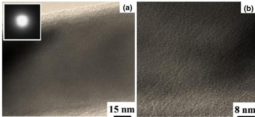
**Fig. 2** HRTEM images of the ZnO NWs irradiated by 1 MeV  $H^+$  ion beam at the doses of  $3 \times 10^{15}$  ion/cm<sup>2</sup> at room temperature. The *inset* is the corresponding SAED image
