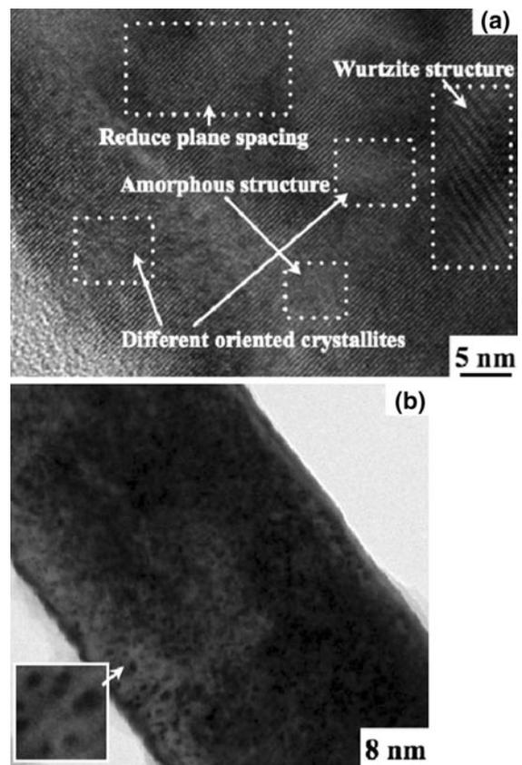
**Fig. 6** HRTEM images of the ZnO NWs irradiated by 1 MeV  $\text{P}^+$  ion beam at room temperature at the doses of **a**  $1 \times 10^{15}$  ion/cm<sup>2</sup> and **b**  $5 \times 10^{15}$  ion/cm<sup>2</sup>
