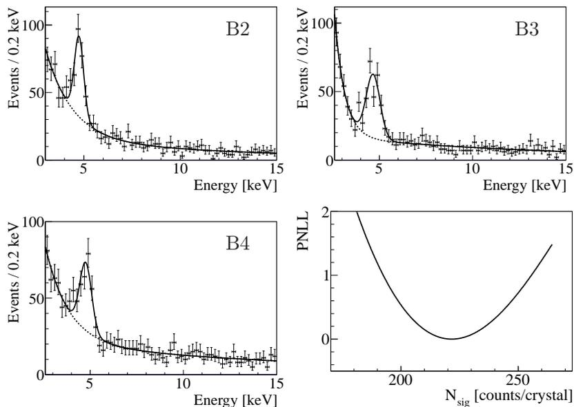
**Figure 6.** Best fits at the 4.7 keV line on the three bolometers with low threshold. On the bottom right, the combined profile negative log-likelihood projected over the number of signal events.
