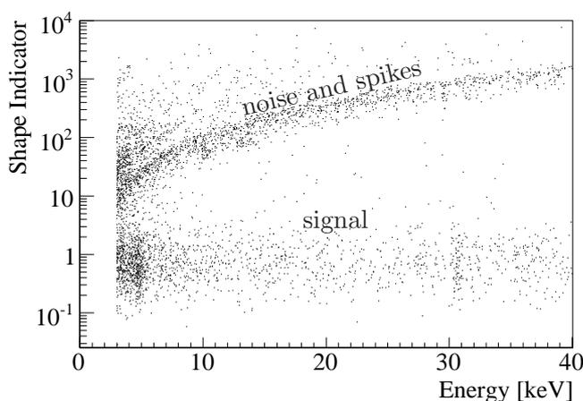
**Figure 4.** Pulse shape indicator (SI) distribution on B2. The band at low SI is populated by signal events. At higher values there are triggered mechanic vibrations, electronic spikes and pileups. The optimal cut for this bolometer was found to be  $SI < 2.2$ .
