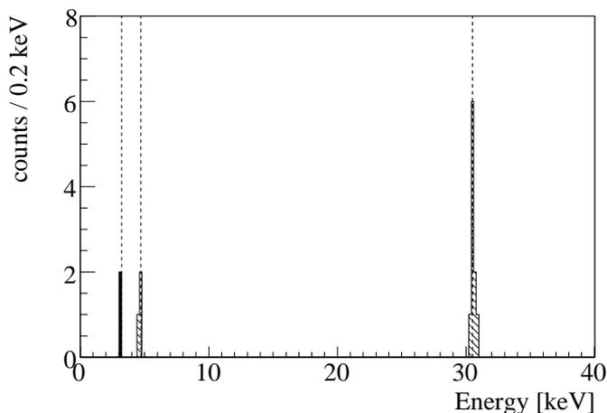
**Figure 3.** Summed energy spectrum from B2, B3 and B4 in time coincidence with an energy deposition on another bolometer (including B1) compatible with the  $\gamma$  lines from  $^{40}\text{K}$  (solid) or  $^{121}\text{Te}$  decays (hashed). The dashed lines represent the nominal values of the de-excitation energies. No event is observed away from these lines.
