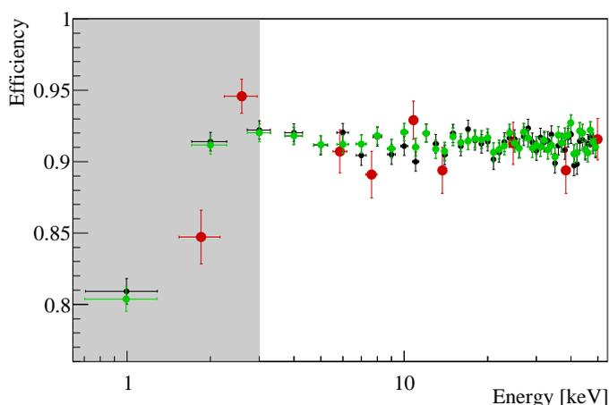
**Figure 1.** Detection efficiency on B2: particle Monte Carlo in black circles, heater Monte Carlo in green circles, heater scan data in big red circles. The shadowed band represents the region below the energy threshold chosen for the data analysis.
