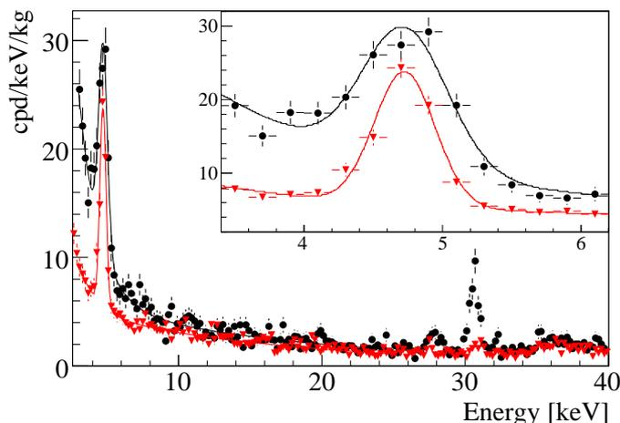
**Figure 8.** Comparison of CCVR2 (black circles) and CUORICINO (red triangles) data, with a zoom on the 4.7 keV. Unlike in CCVR2, CUORICINO data are not corrected for the efficiencies and the calibration at low energies is not optimized.
