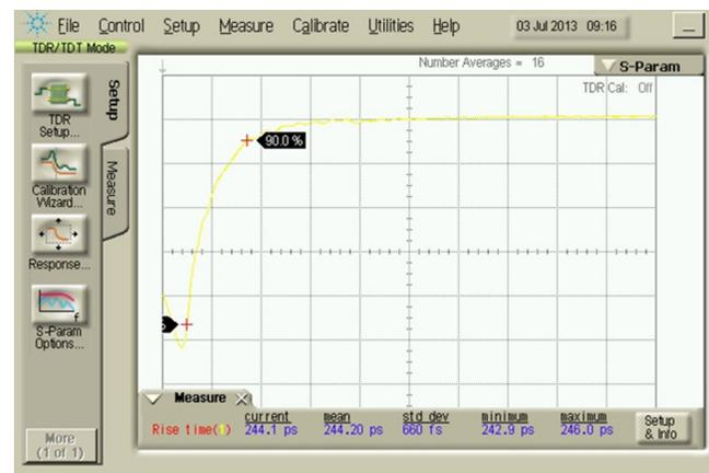
FIG. 12. The rise time of the open-circuit BPM.
