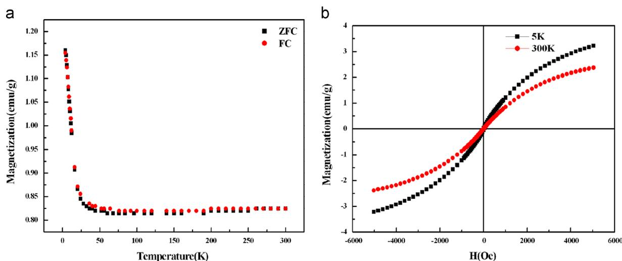
**Fig. 4.** (a) Temperature dependence of the magnetization  $M(T)$  curves of the Co-doped SiC sample for ZFC and FC under 1000 Oe.  $M-H$  curves of the sample measured at 5 and 300 K, respectively.
