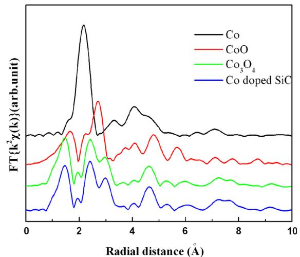
Fig. 3. FT curves of Co K-edge EXAFS oscillation functions  $k^3\chi(k)$  for the Co-doped SiC sample and metallic Co, CoO and Co<sub>3</sub>O<sub>4</sub>, respectively.
