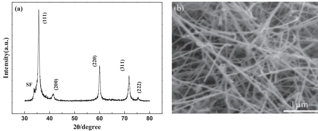
Fig. 1. (a) XRD pattern of Co-doped 3C-SiC nanowires sample and (b) a representative FESEM image of the sample.
