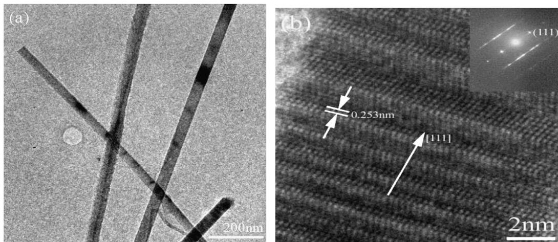
Fig. 2. Images of the Co-doped SiC nanowires: (a) low-magnification TEM image and (b) single nanowire, typical SAED pattern and HRTEM image.
