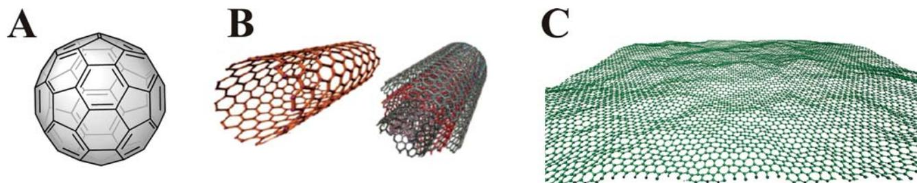
**Fig. (1).** Classic carbon nanomaterials: **A)** buckminsterfullerene C 60 (fullerene-C60). (Reprinted with permission from [14]). **B)** single-walled carbon nanotube. (Reprinted with permission from [15]). **C)** graphene. (Reprinted with permission from [16]). Copyright (2013) American Chemical Society.
