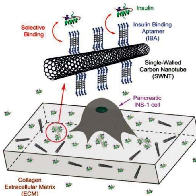
**Fig. (2).** Schematic illustration of optical nanosensor based on CNTs, to measure insulin in pancreatic INS-1 cells *in situ* and in real time. Reprinted with permission from [77]. Copyright (2011) American Chemical Society.
