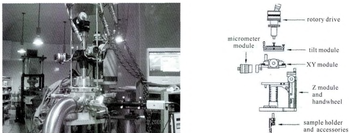
Fig. 5 Photo and schematic diagram of six axis manipulator
