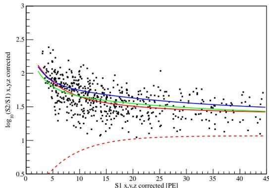
FIG. 3. The comparison of  $^{252}\text{Cf}$  neutron calibration data with the median from the original NEST model (blue line) and the tuned model (green line). A fit to the median of the data is given by the red line. The dashed red line is the NR 99.99% acceptance line based on the tuned MC model.
