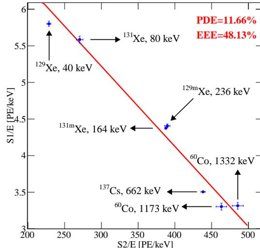
FIG. 2. Linear fit in  $S2/E_{ee}$  vs.  $S1/E_{ee}$  for all  $\gamma$  peaks. Each  $\gamma$  peak was fit with a 2-D Gaussian in the (S1, S2) plane with anti-correlation taken into account; only fit uncertainties are reflected on the data points.
