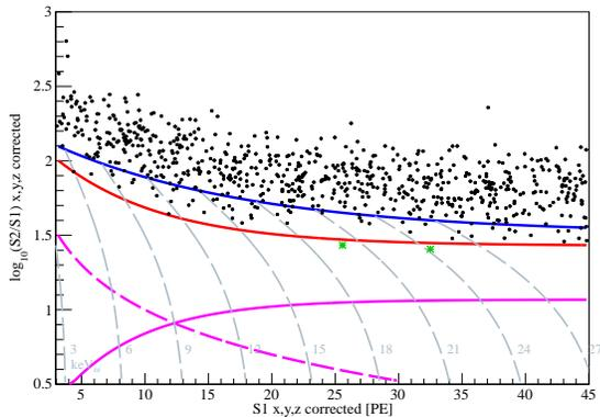
FIG. 5. The distribution of  $\log_{10}(S2/S1)$  versus  $S1$  for dark matter search data. The median of the NR calibration band is indicated as the red curve. The dashed magenta curve is the equivalent 100 PE cut on  $S2$ . The solid magenta and blue curves are the 99.99% and 33.3% NR acceptance curves, respectively. The grey dashed curves are the equal energy curves with NR energy indicated in the figures. The two data points located below the NR median curve are highlighted in green stars.
