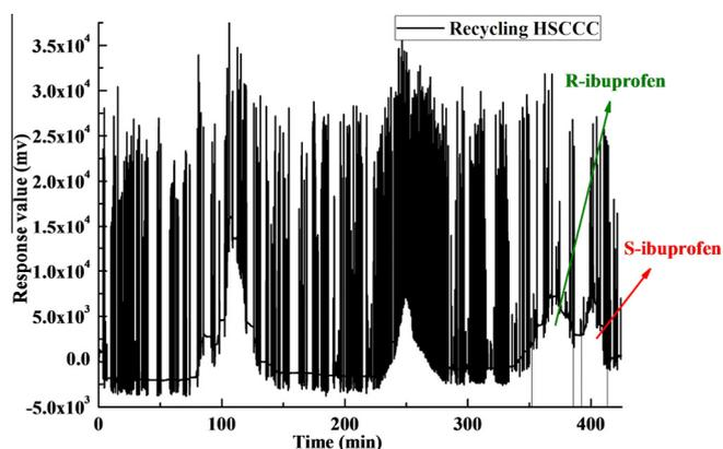
Figure 4. High-speed counter-current chromatography (HSCCC) chromatogram of ibuprofen enantiomers (high-speed counter-current chromatography conditions: revolution speed: 850 rpm; sample loading: 100 mg; detection wavelength: 254 nm; flow rate: 1.2 mL/min; separation temperature: 10 °C; retention of the stationary phase: 53.73%).
