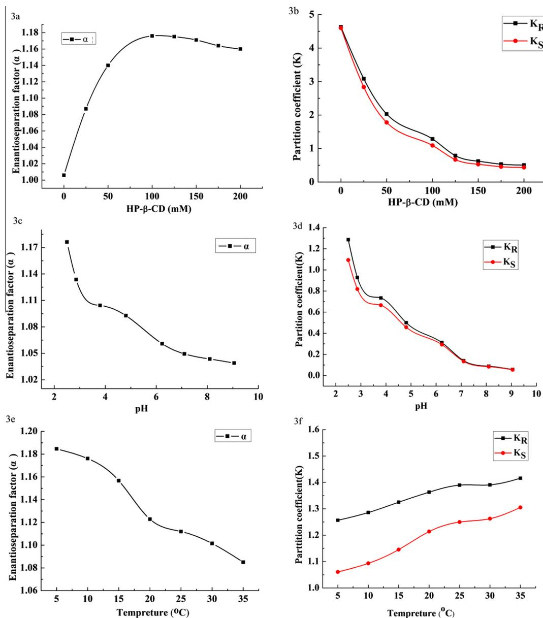
**Figure 2.** Effects of the different parameters (HP- $\beta$ -CD concentration, pH, and temperature) on enantioseparation factors and  $K$ -values for ibuprofen enantiomers.
