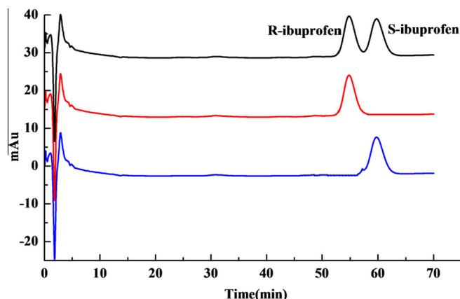
Figure 5. HPLC chromatograms of peak fractions recovered from chiral high-speed counter-current chromatography separation.
