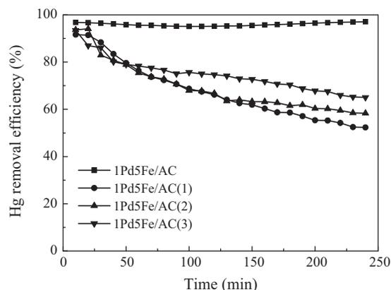
**Fig. 4.** Mercury removal efficiency of 1Pd5Fe/AC sorbent after several recycling (1Pd5Fe/AC: fresh sorbent; 1Pd5Fe/AC(1): sorbent after primary recycling; 1Pd5Fe/AC(2): sorbent after secondary recycling; 1Pd5Fe/AC(3): sorbent after tertiary recycling).
