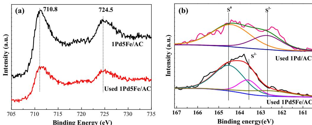
Fig. 7. XPS spectra of (a) Fe 2p and (b) S 2p on the surface of sorbents.
