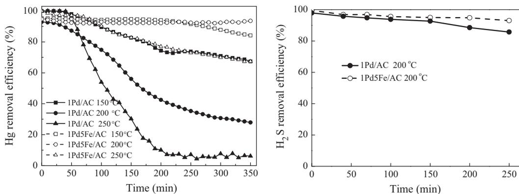
**Fig. 1.**  $\text{Hg}^0$  and  $\text{H}_2\text{S}$  removal efficiency of 1Pd/AC and 1Pd5Fe/AC sorbents at different temperatures. (Reaction conditions:  $40 \mu\text{g}/\text{m}^3$   $\text{Hg}^0$  and 100 ppm  $\text{H}_2\text{S}$  in  $\text{N}_2$ , and  $\text{SV} = 6.4 \times 10^4 \text{ h}^{-1}$ .)
