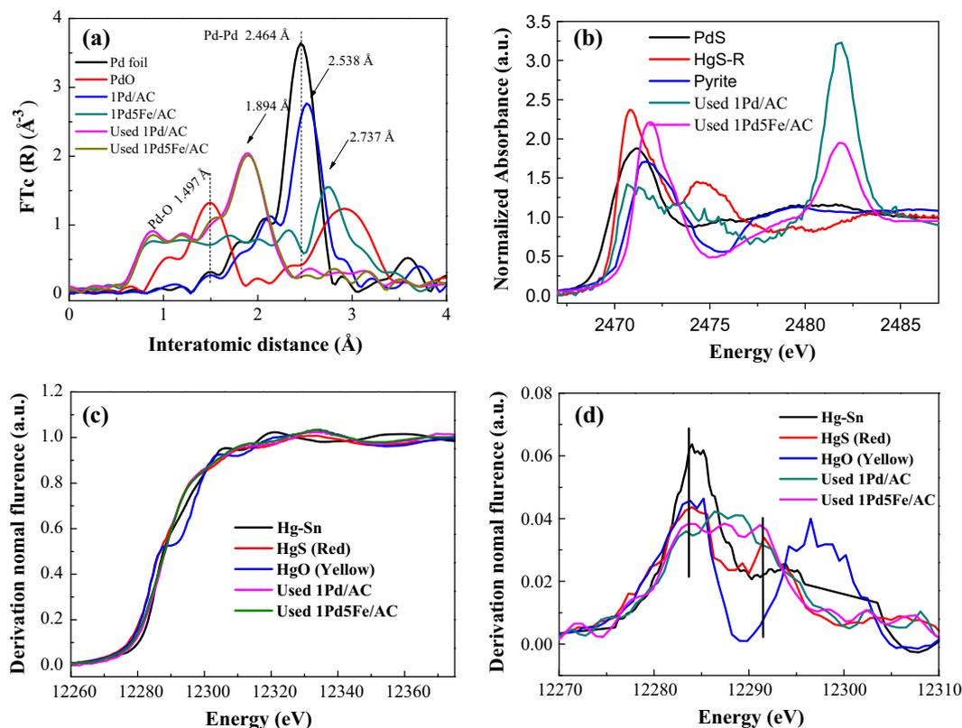
**Fig. 8.** XAS spectra of fresh and used sorbents and reference samples: (a) Pd K-edge EXAFS Fourier transform spectra, (b) S K-edge, (c) Hg L<sub>3</sub>-edge, and (d) the first derivative of the spectra.
