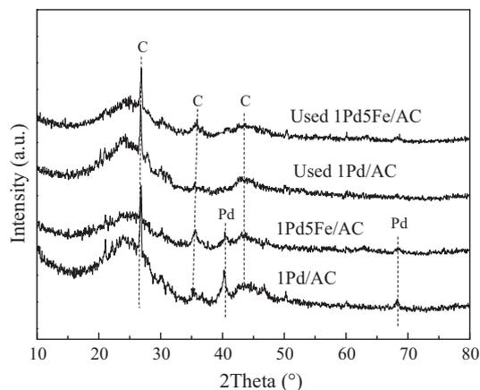
**Fig. 5.** XRD patterns of fresh and used 1Pd/AC and 1Pd5Fe/AC sorbents.
