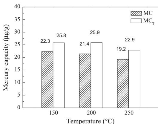
**Fig. 2.** Experimentally determined ( $\text{MC}$ ) and theoretically calculated ( $\text{MC}_T$ ) adsorption mercury capacity of sorbent 1Pd5Fe/AC at different temperature. (Reaction conditions:  $40 \mu\text{g}/\text{m}^3$   $\text{Hg}^0$  and 100 ppm  $\text{H}_2\text{S}$  in  $\text{N}_2$ , and  $\text{SV} = 6.4 \times 10^4 \text{ h}^{-1}$ .)
