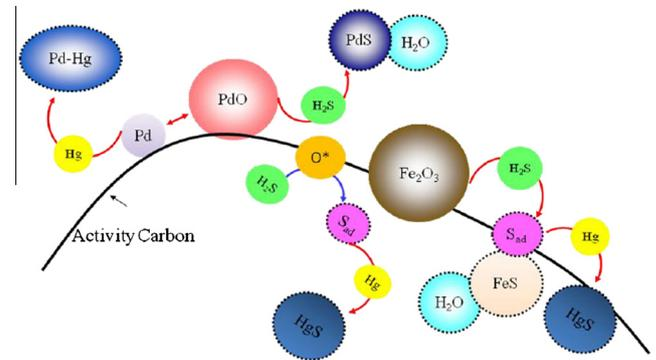
Fig. 9. Possible reactions on the surface of 1Pd5Fe/AC sorbent.
