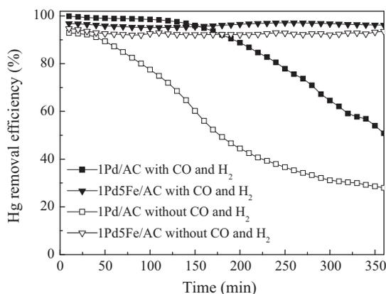
**Fig. 3.** Effects of CO and  $\text{H}_2$  on the  $\text{Hg}^0$  removal efficiencies of 1Pd/AC and 1Pd5Fe/AC sorbents. (Reaction conditions: 200 °C,  $40 \mu\text{g}/\text{m}^3$   $\text{Hg}$ , 100 ppm  $\text{H}_2\text{S}$ , 20 vol% CO, 10 vol%  $\text{H}_2$  in  $\text{N}_2$ , and  $\text{SV} = 6.4 \times 10^4 \text{ h}^{-1}$ .)
