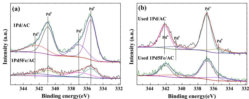
Fig. 6. XPS spectra of Pd 3d on the surface of (a) fresh and (b) used 1Pd/AC and 1Pd5Fe/AC sorbents.
