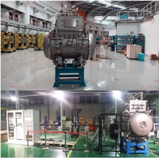
Fig. 6. The 50-period SCU cryostat and the test site.
