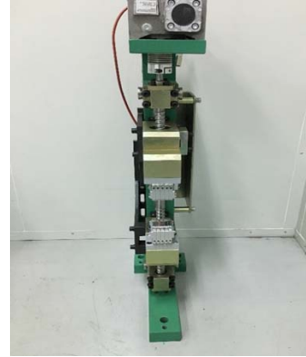
图 3 纯永磁移相器实物图 Fig.3 Photograph of pure permanent magnet phase shifter.
