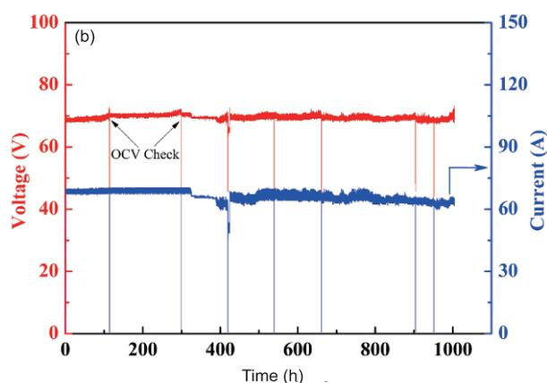
**Figure 2** 5 kW-HTSE system and operation at Shanghai Institute of Applied Physics. (a) Photo of the system; (b) long-term stability test of the system at 750 °C under a current density of 0.25 A/cm<sup>2</sup> (color online).
