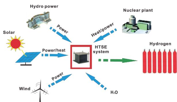
**Figure 1** HTSE system coupled with clean energies for energy storage and hydrogen production (color online).
