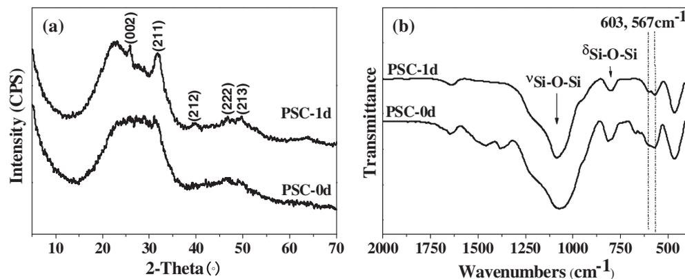
Fig. 4. XRD (a) and FTIR (b) spectra of PSC glasses after immersing in SBF for 1 d.
