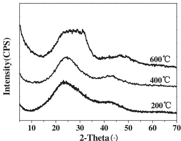
Fig. 2. The XRD spectra of PSC glasses after stabilization at 200 °C, 400 °C and 600 °C.
