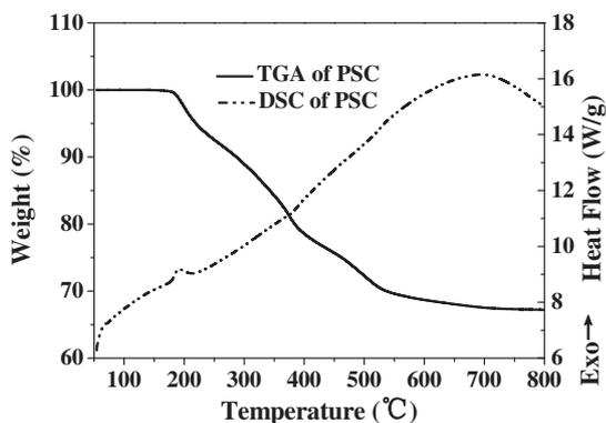
Fig. 1. The TGA-DSC traces of the calcium phosphosilicate gels (PSC:  $(\text{CaO})_{0.35}(\text{SiO}_2)_{0.54}(\text{P}_2\text{O}_5)_{0.11}$ ) after dried at 120 °C.
