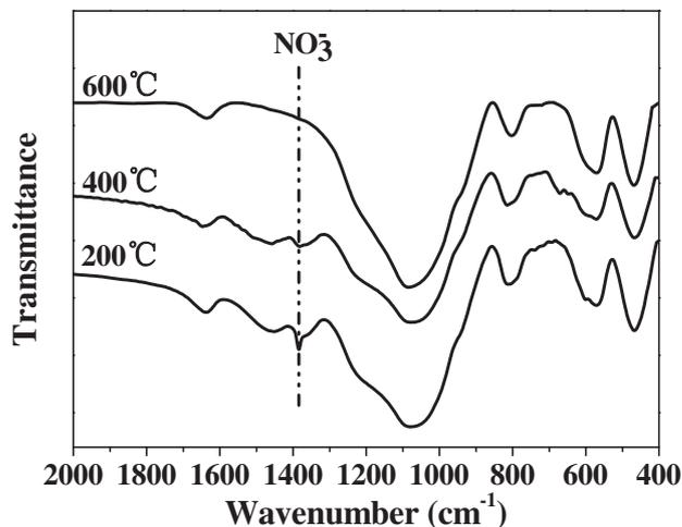
Fig. 3. The FTIR spectra of PSC glasses after stabilized at different temperature.
