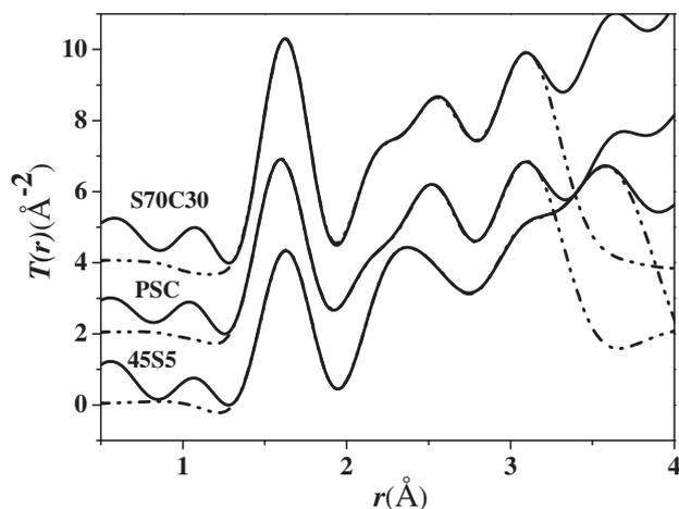
Fig. 5. The real-space data X-ray diffraction patterns of 45S5, S70C30 and PSC glasses, as determined from HEXRD data (solid curves: experimental; dashed curves: NXFIT data).
