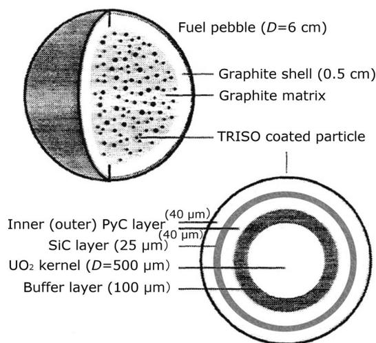
**Fig. 1** TRISO-coated particle (bottom) and fuel pebble (top) [5]
