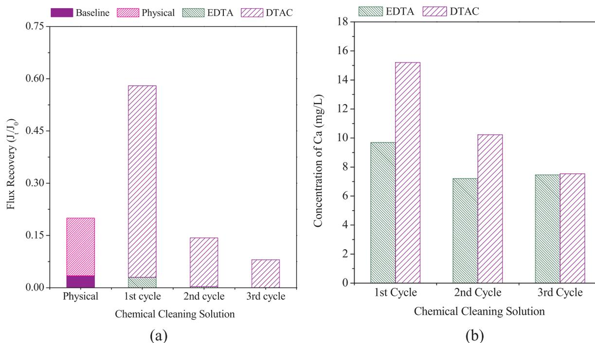
Fig. 4. For EDTA/DTAC cleaning procedure in the bench-scale experiments, (a): flux recoveries, and (b): eluotropic Ca<sup>2+</sup> concentration. The multiple-step cleaning procedure of EDTA/DTAC was continuously repeated three times for one fouled membranes, and its each implement was named the 1st E/D, 2nd E/D and 3rd E/D in sequential. Herein, the concentrations of EDTA and DTAC were 10 and 76 mM, respectively.
