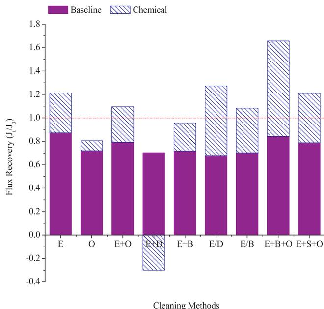
Fig. 7. Flux recoveries for the cleaning methods in the pilot-scale experiments. “/” and “+” represent cleanings with sequential procedures and formulated solutions, respectively. “E”, “D”, “B”, “S”, and “O” represent EDTA, DATC, BS-12, SDBS, and NaClO solutions, respectively, the concentrations of which were 10, 76, 5.56, 4.80 mM and 0.2% (volume percent), respectively.
