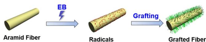
Fig. 1. Modification of Kevlar fibers by EB-induced post-grafting polymerization.
