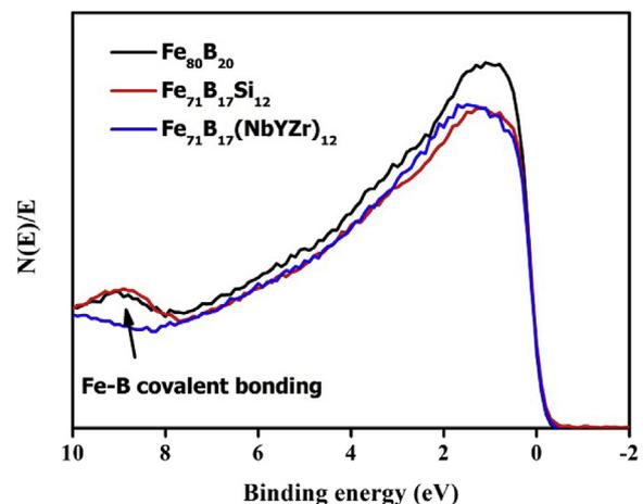
Fig. 5. Electronic structures obtained from XPS measurements: FeB metallic glass is a reference here.
