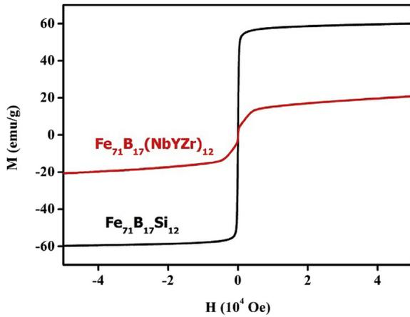
Fig. 3. Room-temperature magnetizations of two Fe-based metallic glasses.
