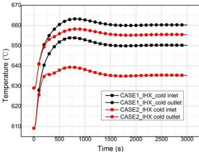
Fig. 16 Temperature variations of secondary coolants in two cases
