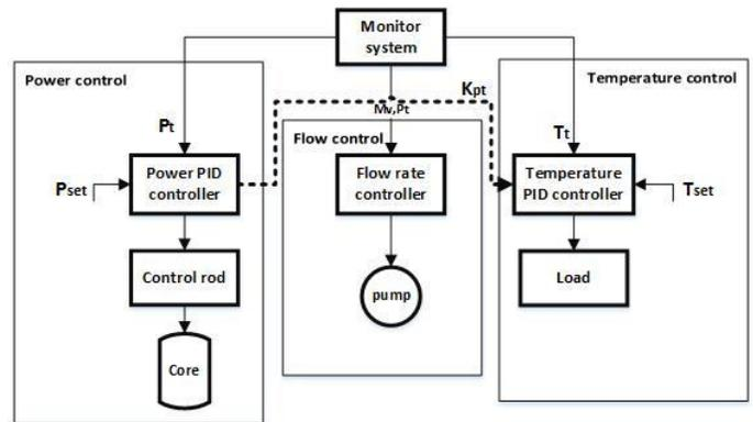
Fig. 5 Structural representation of control scheme
