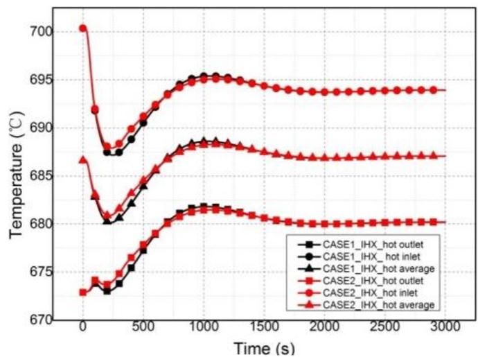
Fig. 15 Temperature variations of primary coolants in two cases
