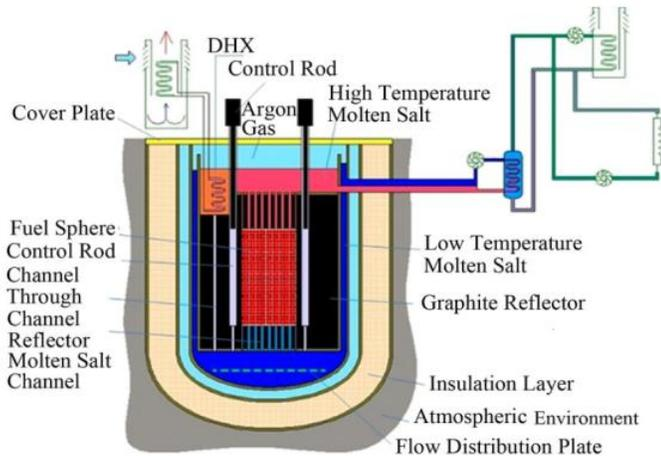
Fig. 1 Schematic diagram of FHER
