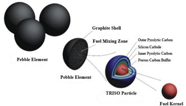
Fig. 2 Diagram of pebble element
