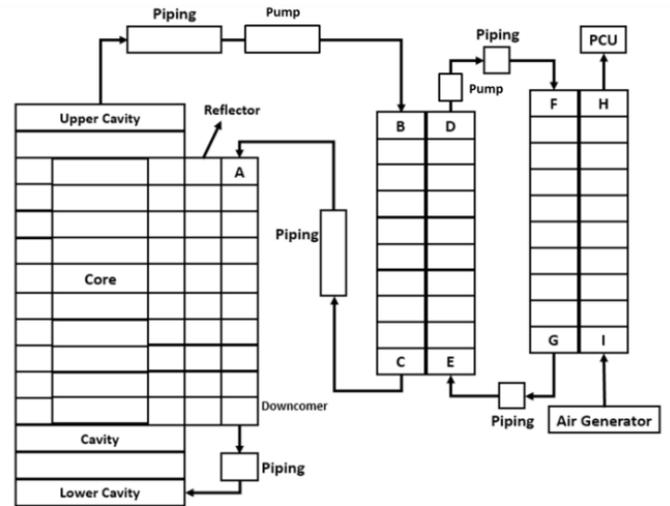
Fig. 3 Node diagram of FHER
