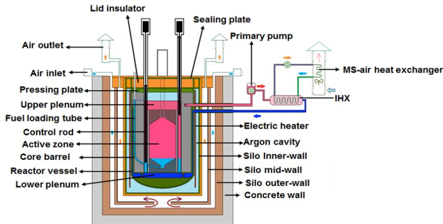
Fig 1. Schematic of TMSR-SF1 reactor system
