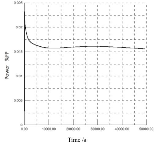
Figure 2 Passive residual heat removal system power
