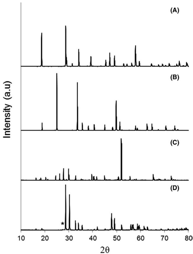
**FIGURE 3** X-ray diffraction patterns of (A)  $\text{CaWO}_4$ , (B)  $\text{YVO}_4$ , (C)  $\text{LaVO}_4$ , and (D)  $\text{YNbO}_4$ . Trace monoclinic  $\text{ZrO}_2$  is indicated by the star in (D). Otherwise, the ceramics are essentially phase pure at the level of detection typical for laboratory X-ray diffraction. The pattern shown for  $\text{LaVO}_4$  appears to show the effects of preferred orientation in the powder sample
