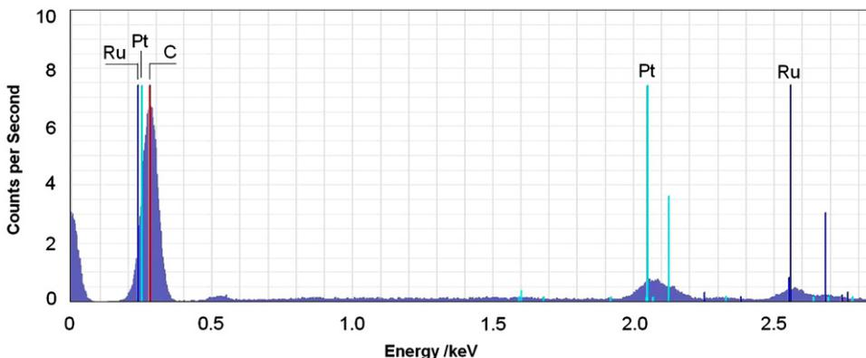
Fig. 2. EDX spectrum of the Pt/Ru nano-particles on MWCNTs.
