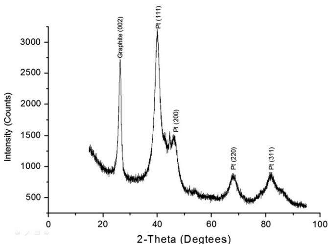
Fig. 3. XRD patterns of radiation synthesized PtRu/CNT catalysts.
