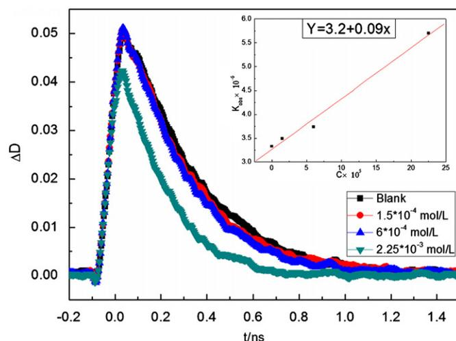
**Fig. 5.** Decay curves of hydrated electron for solutions with different concentrations of Pt(IV) added with surfactant of 0.5%. The inset: the rate constants vs concentrations.
