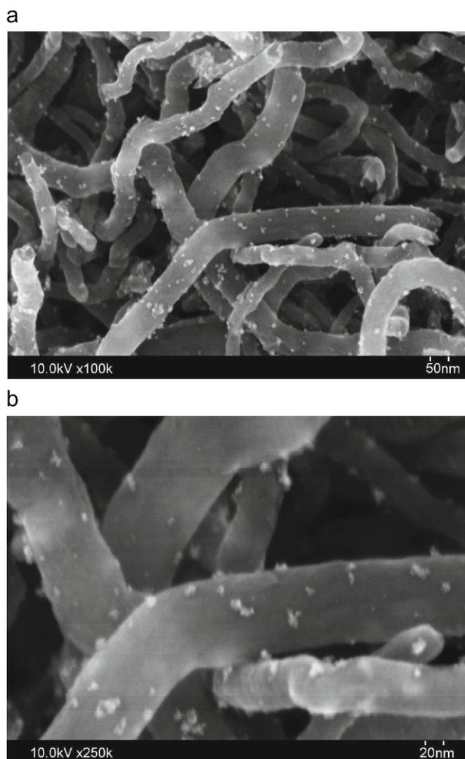
Fig. 1. SEM image of the Pt/Ru nano-particles on MWCNTs prepared in aqueous solution with a water/iso-propanol ratio of 60:40(v/v) irradiated to 40 kGy.
