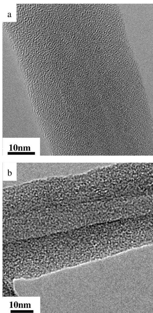
**Fig. 3.** HRTEM images of MWCNTs irradiated with 70 keV proton beams at doses of (a)  $1 \times 10^{17}$  and (b)  $1 \times 10^{18}$  protons/cm<sup>2</sup>.
