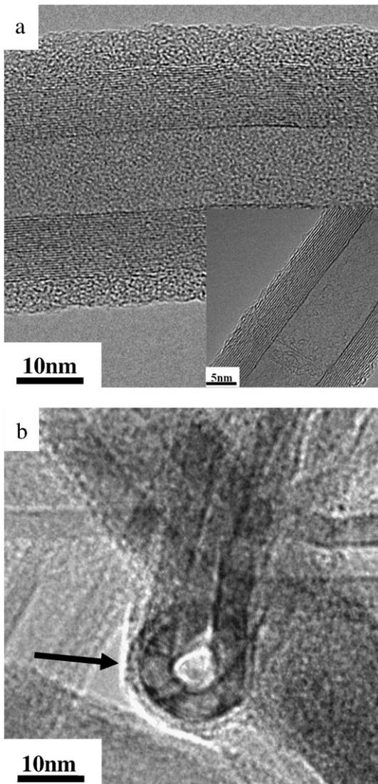
**Fig. 1.** (a) HRTEM image of a MWCNT irradiated with a 70 keV proton beam at a dose of  $5 \times 10^{16}$  protons/cm<sup>2</sup>. The inset shows the HRTEM image of an as-grown MWCNT. (b) Cross-sectional TEM image at a slightly tilted angle. The amorphous structure of the MWCNT is denoted by the arrow.
