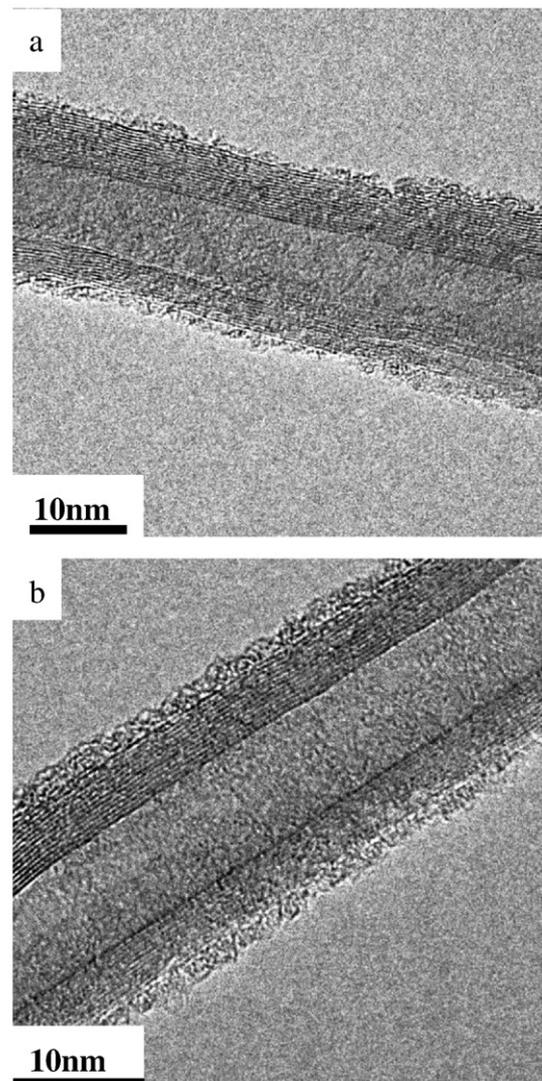
**Fig. 2.** HRTEM images of MWCNTs irradiated with 70 keV proton beams at doses of (a)  $1 \times 10^{15}$  and (b)  $5 \times 10^{15}$  protons/cm<sup>2</sup>.
