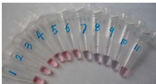
Fig. 2 Color change of gold nanoprobe upon being treated with pure water (1) and a series of metal ions of 100 \mu\text{M} , i.e. , \text{Pb}^{2+} , \text{Cd}^{2+} , \text{Cu}^{2+} , \text{Mn}^{2+} and \text{Zn}^{2+} (2–6). Tubes 7–11 show the concentration profile for the \text{Hg}^{2+} -induced color change of gold nanoprobe (from left to right: 100 \mu\text{M} , 50 \mu\text{M} , 25 \mu\text{M} , 10 \mu\text{M} and 5 \mu\text{M} ). In all these experiments, \text{NaClO}_4 of 2.25 M was added to tubes after 5-min incubation.
