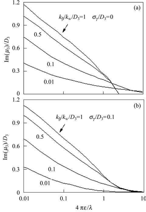
Fig. 1. Scaling function for the 3rd linear harmonic gain vs. scaled emittance for several values of  $k_\beta/k_w/D_3$ , corresponding to scaled energy spread (a)  $\sigma_\gamma/D_3 = 0$  and (b)  $\sigma_\gamma/D_3 = 0.1$  with the optimal detuning.
