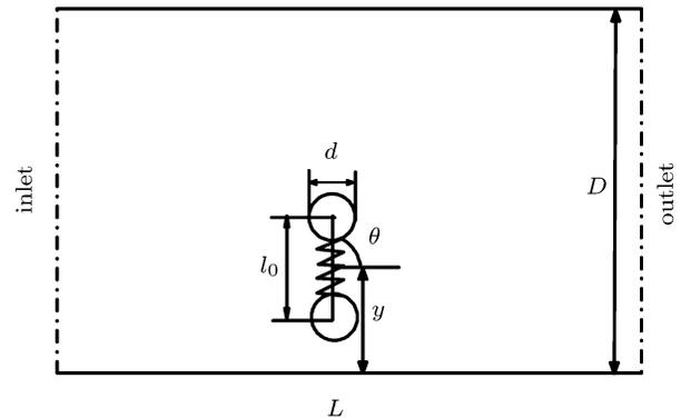
**Fig.1.** Schematic diagram of a neutrally buoyant dumbbell moving in a Poiseuille flow.
