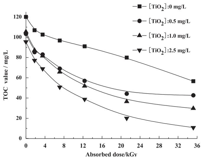
Fig. 3. The relationship between TOC value and absorbed dose with different  $\text{TiO}_2$  contents.
