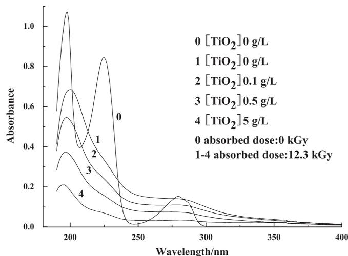
Fig. 1. Absorption spectra of 1 mmol L<sup>-1</sup> 4-chlorophenol aqueous solutions with different TiO<sub>2</sub> contents by 12.3 kGy electron beam irradiation (curve 0 before irradiation). [TiO<sub>2</sub>](g L<sup>-1</sup>): 0 (curves 0 and 1), 0.1 (curve 2), 0.5 (curve 3) and 5 (curve 4).
