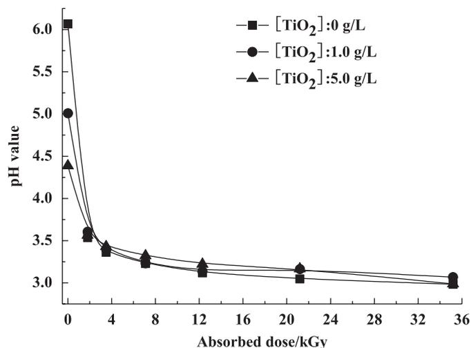
Fig. 4. The change of pH value with absorbed dose with different  $\text{TiO}_2$  contents.
