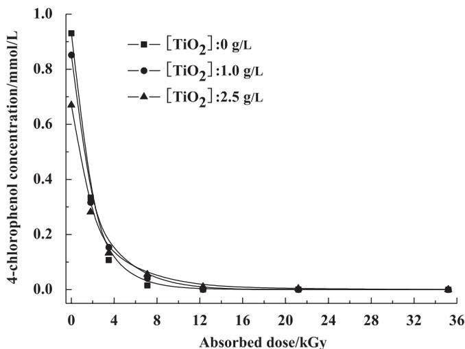
Fig. 2. The relationship between 4-chlorophenol concentration and absorbed doses with different  $\text{TiO}_2$  contents.
