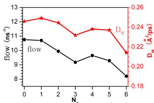
**Figure 2.** Water flow and one-dimensional diffusion coefficient  $D_w$  of water molecules inside the channel with respect to the number of 5/7 pair defects  $N_d$ .
