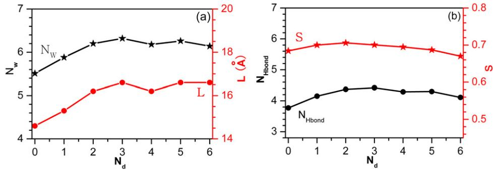
**Figure 3.** (a) Average number of water molecules  $N_w$  inside the nanotube together with the length of nanotube  $L$  with respect to the number of 5/7 pair defects  $N_d$ . (b) Average number of hydrogen bonds  $N_{\text{Hbond}}$  inside the nanotube and  $S = N_{\text{Hbond}}/N_w$  in different model systems.
