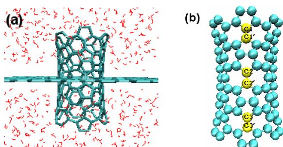
**Figure 1.** (a) Snapshot of the simulation systems. A (6, 6) single-walled carbon nanotube with triple 5/7 pair defects together with the graphite sheet are dissolved in water. (b) C1–C1', C2–C2' and C3–C3' are rotated by 90°, forming triple 5/7 pair defects in the nanotube.
