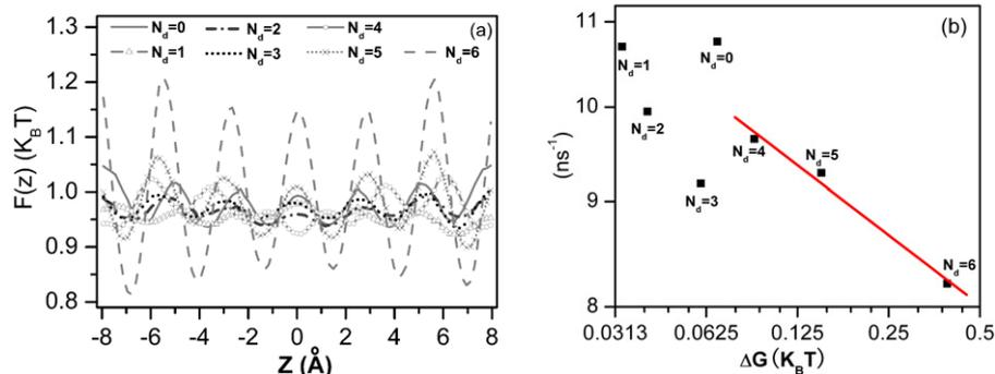
**Figure 4.** (a) Potential of mean force (PMF) profiles of water molecules inside channel along the  $z$ -direction in different systems. (b) The relationship of flow to the height of the barrier,  $\Delta G$ , in PMF profiles. When  $N_d > 3$ , the data can be fitted by a power law flow =  $7.4 \times \Delta G^{-0.11}$ .
