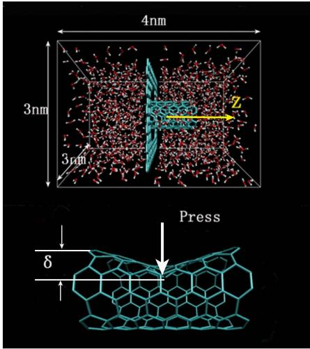
FIG. 1. (Color online) Snapshot of the simulation system. The CNT and the graphite sheet are solvated in a box ( $3 \times 3 \times 4 \text{ nm}^3$ ) with 1036 water molecules. The nanotube of the simulation setup is amplified. An external force, marked by press, acts on an atom of the carbon nanotube and a deformation can be clearly seen.  $\delta$  is the displacement of the forced atom from its initial equilibrium position.
