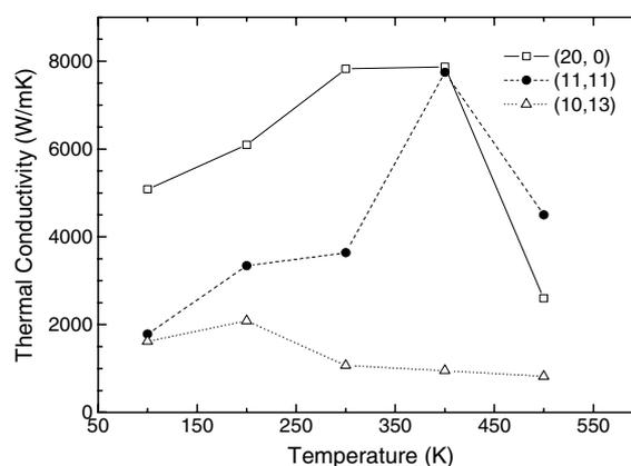
**Figure 4.** Thermal conductivities of (20, 0)—open squares, (11, 11)—solid circles, and (10, 13)—open triangles, nanotubes.
