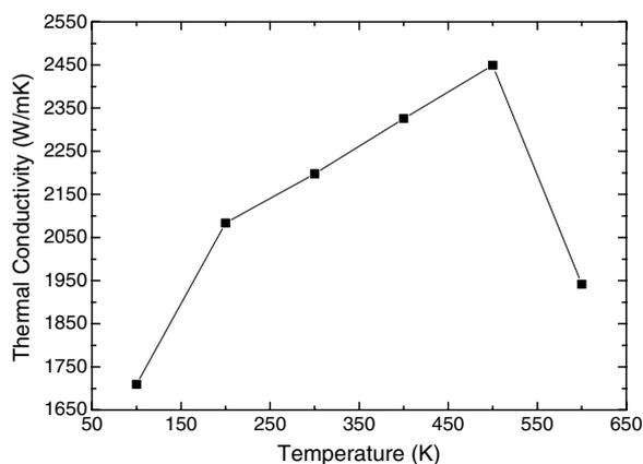
**Figure 3.** Thermal conductivities of a (10, 10) nanotube.
