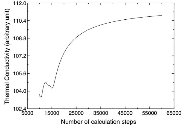
**Figure 2.** The converging behaviour of the thermal conductivity of a (11, 11) nanotube with increasing number calculation steps, for  $F_e = 0.3 \text{ \AA}^{-1}$ , at temperature  $T = 300 \text{ K}$ .
