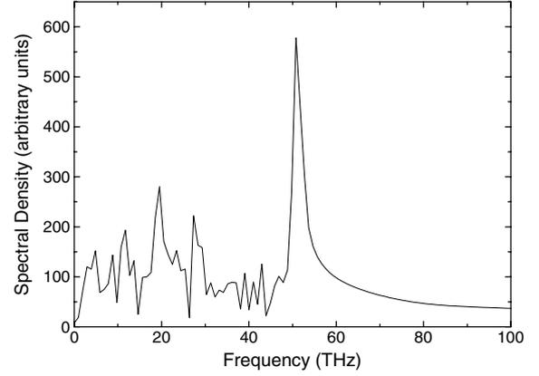
**Figure 1.** Phonon spectrum of the (10, 10) nanotube calculated from the Fourier transform of the velocity auto-correlation function generated during the simulations.
