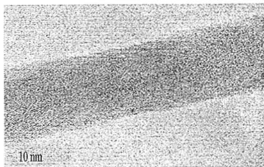
Fig.1 TEM image of MWNTs irradiated to 250kGy by ^{60}\text{Co} \gamma -rays
