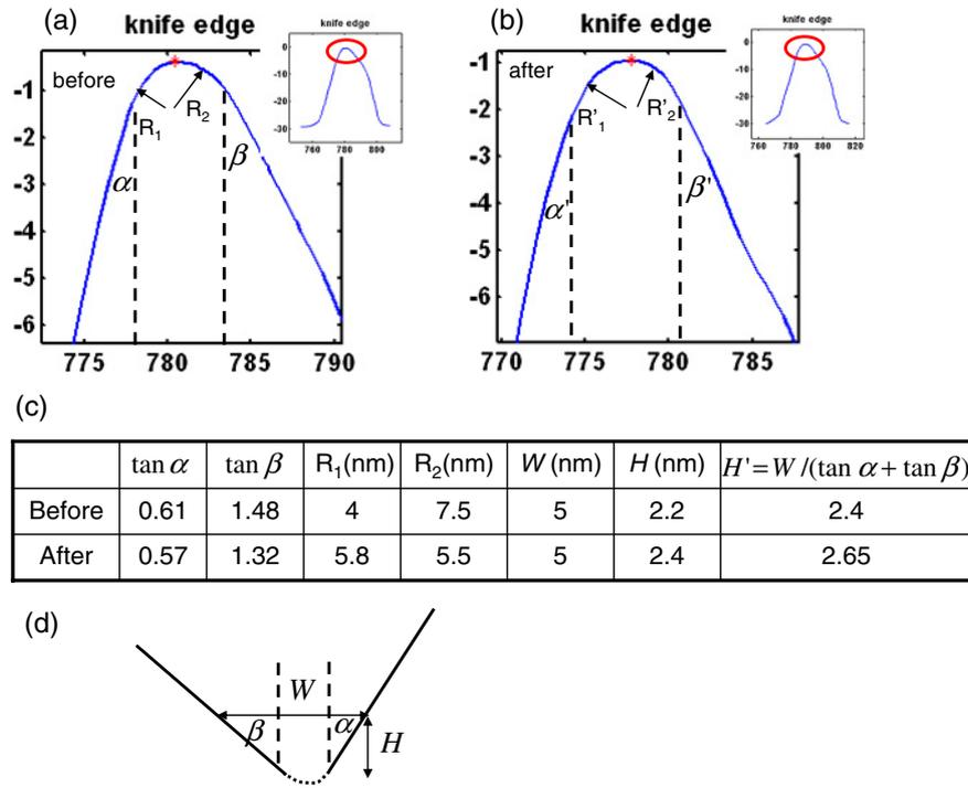
Fig. 3. (Color online) Extracted parameters from the top of the probe tip and a constructed tip model. (a) Tip shape before the CNT imaging experiment; (b) tip shape after the CNT imaging experiment; (c) table listing the four parameters ( $\alpha$ ,  $\beta$ ,  $R_1$ ,  $R_2$ ) extracted from (a) and (b) to describe the tip, as well as  $W$ ,  $H'$  and  $H$ ; (d) model of the extracted tip shape without knife edge convolution effects.
