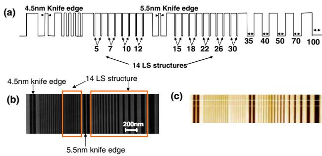
Fig. 1. (Color online) The AFM probe tip characterizer. (a) Schematic of the characterizer showing lattice feature sizes as measured by TEM; (b) SEM image of the tip characterizer; (c) AFM image of the tip characterizer, acquired with a conventional probe tip.
