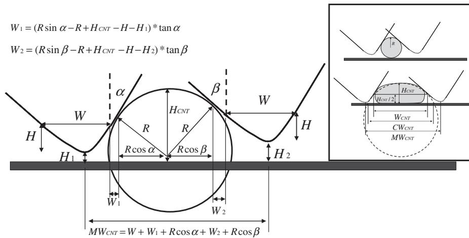
Fig. 6. Schematic drawing of the spherical CNT size-correction model.
