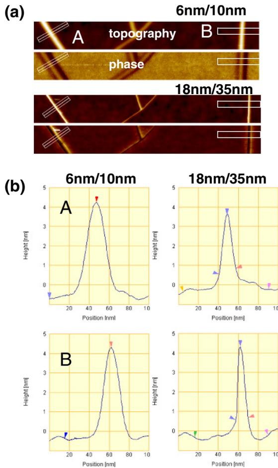
Fig. 4. (Color online) AFM images (topography and phase) of CNTs and their corresponding line profiles. (a) AFM images of CNTs acquired with different oscillation ratios ( $A_{sp}/A_0$ ), denoted above the images; (b) line profiles of the two CNTs marked in (a).
