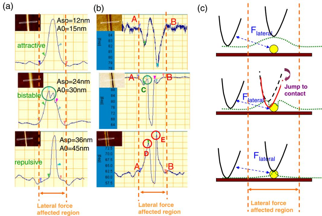
Fig. 5. (Color online) Contact point judgment as determined from dynamic mode AFM of a single CNT. (a) Line profiles of the topography image of the CNT acquired with three sets of oscillations (listed in the figure); (b) corresponding phase images and linescans; (c) schematic drawings of tip movement as deduced from the results of the three imaging conditions used in (a) and (b).
