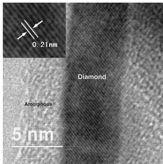
Fig. 3. HRTEM image of the crystalline diamond core and amorphous carbon sheath. The inset shows the (111) planes with a spacing of 0.21 nm.
