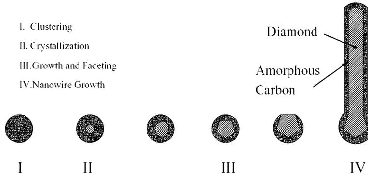
Fig. 4. The proposed model for the formation of nanodiamond and the growth of diamond nanorods under hydrogen plasma irradiation of MWCNTs at high temperature. Amorphous carbon clusters formed in the step I. The crystallization of diamond began in the core of carbon clusters (step II) followed by the diamond growth and faceting stage (step III). After the diamond nanocrystallites were faceted, diamond nanorods began to grow at the nanorod tips (step IV).
