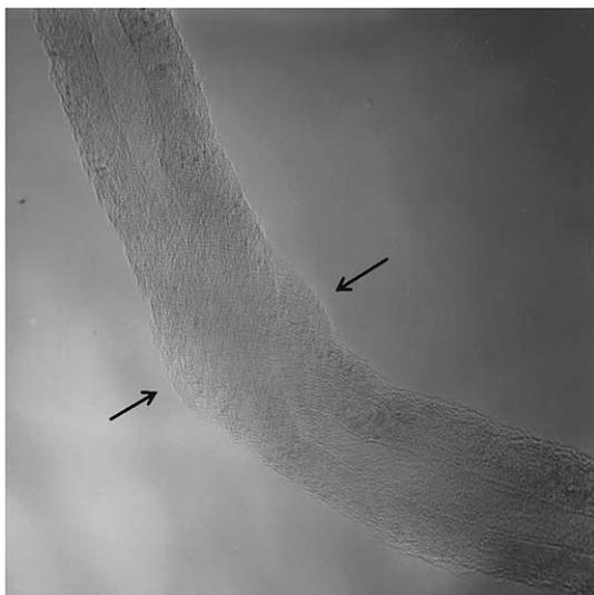
Fig. 1. TEM image of electron beam irradiated MWCNTs.
