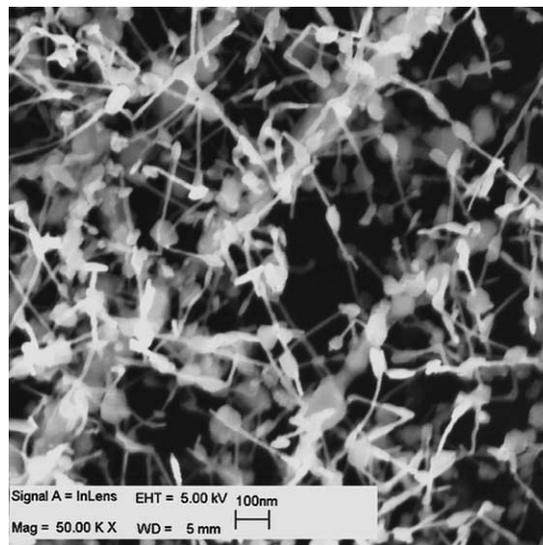
Fig. 2. SEM image of carbon nanorods after hydrogen plasma treatment of MWCNTs for 20 h.
