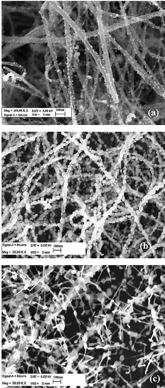
Fig. 2. SEM image of hydrogen plasma treatment of MWCNTs at temperature of 1000 K for 4 h (a), 10 h (b) to form chain-like DNWs and 20 h (c) to form single-crystal DNWs.
