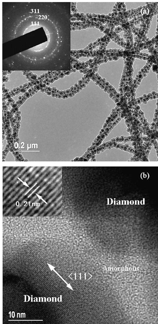
Fig. 1. (a) Low magnification TEM image of chain-like DNWs from the MWCNTs after hydrogen plasma treatment at temperature of 1000 K for 10 h. The ring pattern in the inset from electron diffraction confirmed the diamond structure of nanocrystallines. (b) HRTEM image shows the diamond (111) lattice planes with a  $d$ -spacing of 0.21 nm. The inset is the simulated image of the nanocrystals after image filter processing by Fourier transform.
