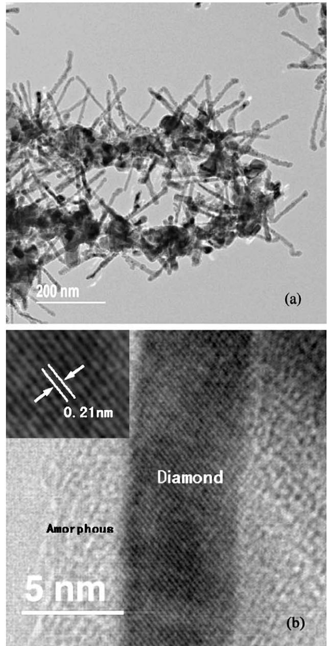
Fig. 3. (a) TEM image of the single-crystal DNWs from the MWCNTs after treatment in hydrogen plasma at temperature of 1000 K for 20 h. (b) High-resolution TEM image shows the structure of single-crystal DNWs with crystalline core and amorphous carbon sheath. The inset is the simulated image of the nanocrystals after image filter processing by Fourier transform.
