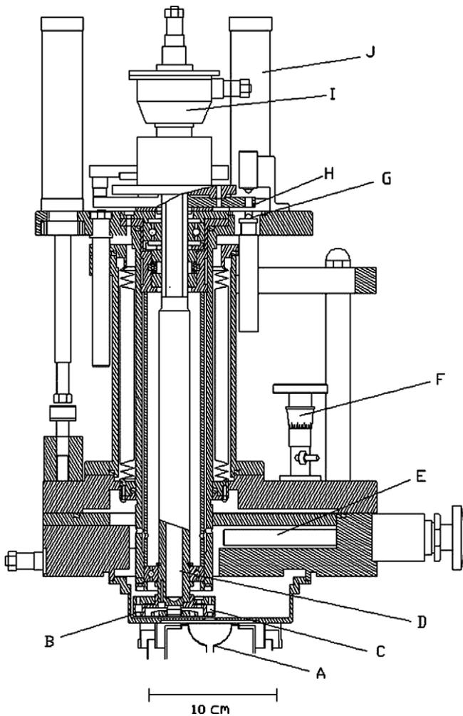
Fig. 2. Schematic side view of the SMCAMS multi-cathode device. A: ionizer; B: cathode wheel; C: sample holder ( $-15.0$  to  $-17.5$  kV); D: rotary shaft; E: gate valve; F: pinhole valve; G: positioning bolt; H: ratchet wheel; I: coolant head and J: gas cylinder.
