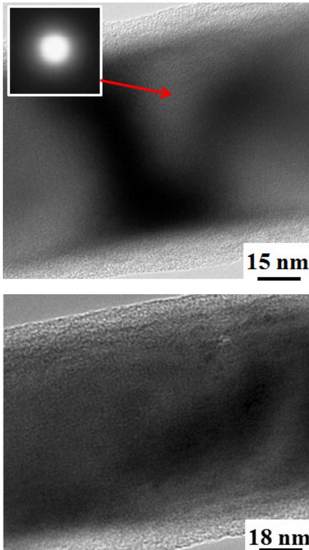
Fig. 4. TEM image of the ZnO NWs after irradiation with  $H^+$  beam with an intensity of  $2 \times 10^{17}$  ions/cm<sup>2</sup>. The inset is the corresponding SEAD image showing that the amorphous structure has dominated the whole nanowire.
