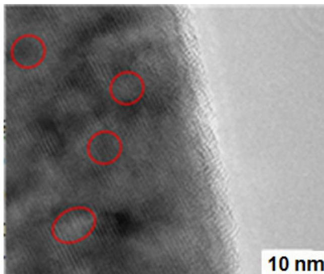
Fig. 2. After irradiation with a proton beam of  $5 \times 10^{15}$  ions/cm<sup>2</sup>. Nanosized defects start to form on the crystal lattice (marked with red circles) (color online).
