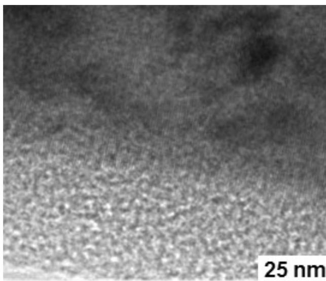
Fig. 3. After irradiation with a proton beam of  $1 \times 10^{17}$  protons/cm<sup>2</sup>. Nanosized defects start to agglomerate to form a bigger area of the amorphous region.
