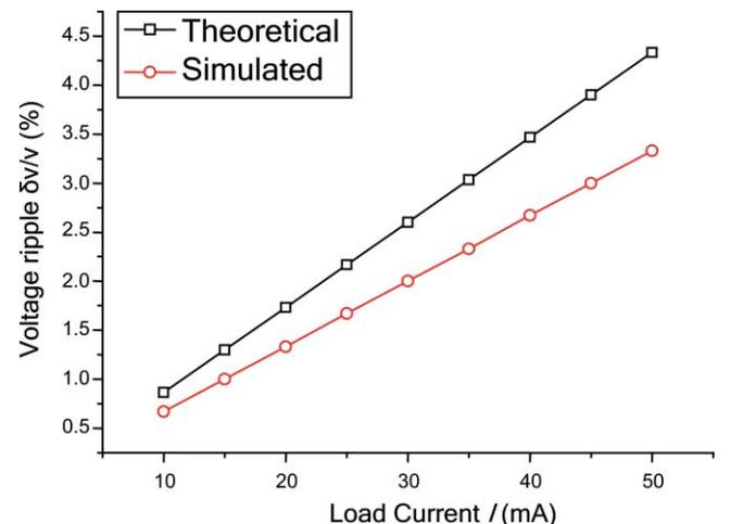
FIG. 3. (Color online) Voltage ripple vs load current current of SCW generator.
