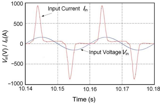
FIG. 9. (Color online) Input voltage and current waveforms.
