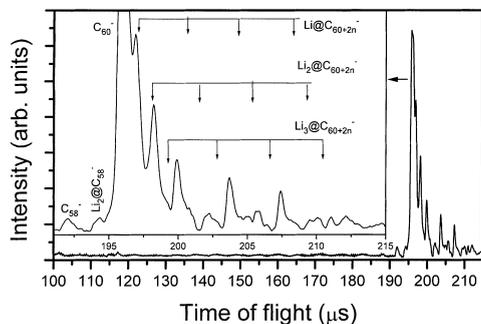
Fig. 3. Time-of-flight mass spectrum of negatively charged ions for the film deposited with a collision energy of 30 eV of  $\text{Li}^+$  ion beam.
