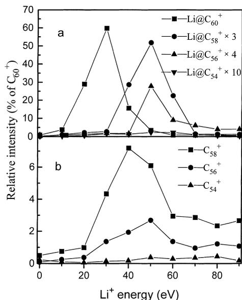
Fig. 2. Dependence of intensities of lithium endohedral fullerene ions (a) and fragments ions (b) relative to C<sub>60</sub><sup>+</sup> with collision energy.
