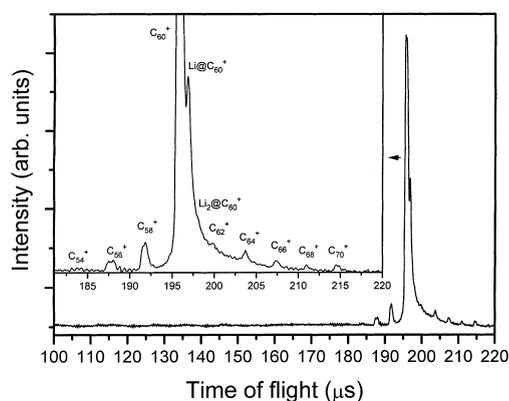
Fig. 1. Time-of-flight mass spectrum of positively charged ions for the film deposited with a collision energy of 30 eV of  $Li^+$  ion beam.
