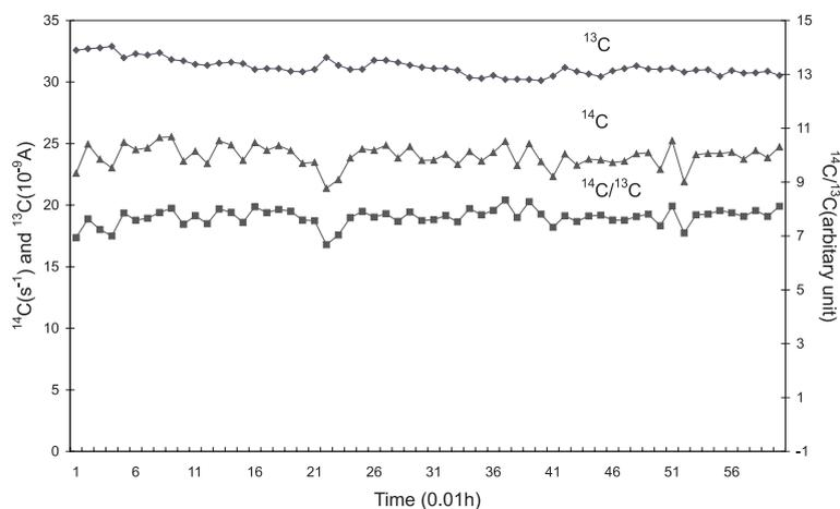
Fig. 4.  $^{13}\text{C}$ ,  $^{14}\text{C}$  and  $^{14}\text{C}/^{13}\text{C}$  versus cycle number during A-sequential acceleration, where the maximum  $^{14}\text{C}$  counting rate reached is about 25 cps measured in 60 cycles with each 40 s by consecutively rotating samples three times.
