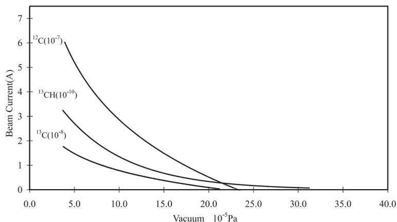
Fig. 5. Beam current of  $^{12}\text{C}$ ,  $^{13}\text{C}$  and  $^{13}\text{CH}$  versus vacuum in the SMCAMS.
