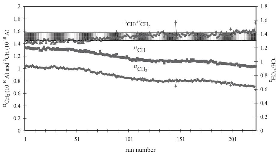
Fig. 2.  $^{13}\text{CH}$ ,  $^{12}\text{CH}_2$  and  $^{13}\text{CH}/^{12}\text{CH}_2$  versus cycle number during  $F$ -sequential acceleration.
