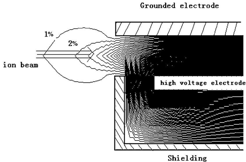
Fig. 6. The calculated distribution of the electric potential penetrating from the exit (entrance) of the horizontal injection (extraction) deflector with full shielding.
